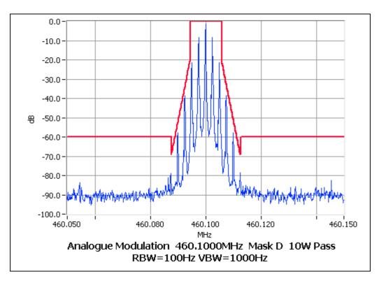
NAME OF TEST: OCCUPIED BANDWIDTH FFSK
