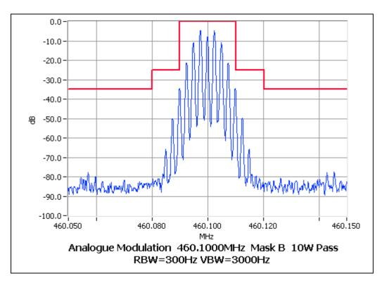
NAME OF TEST: OCCUPIED BANDWIDTH FFSK
