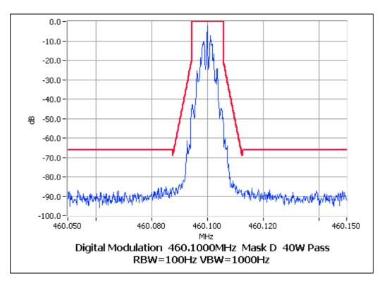
NAME OF TEST: OCCUPIED BANDWIDTH FFSK
