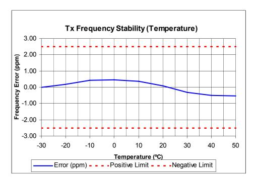
Tx FREQUENCY: 460.1 MHz 40 W 25.0 kHz channel Spacing
