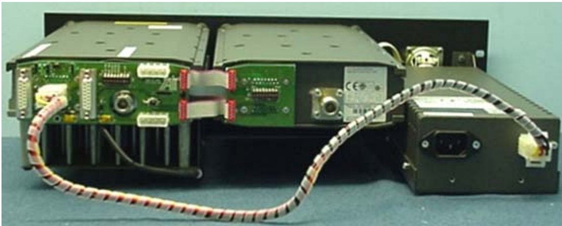
Overall external view rear (Transmitter, Receiver, Power Supply)
