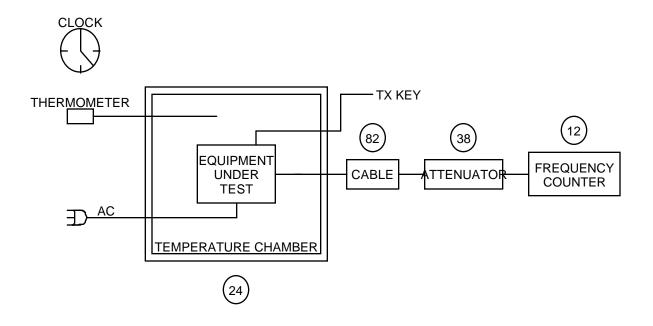
NAME OF TEST: TRANSMITTER FREQUENCY STABILITY (TEMPERATURE)
