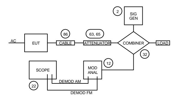
NAME OF TEST: TRANSIENT FREQUENCY BEHAVIOUR
