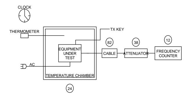
NAME OF TEST: TRANSMITTER FREQUENCY STABILITY (TEMPERATURE)
