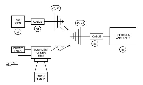
NAME OF TEST: SPURIOUS EMISSIONS (RADIATED)
