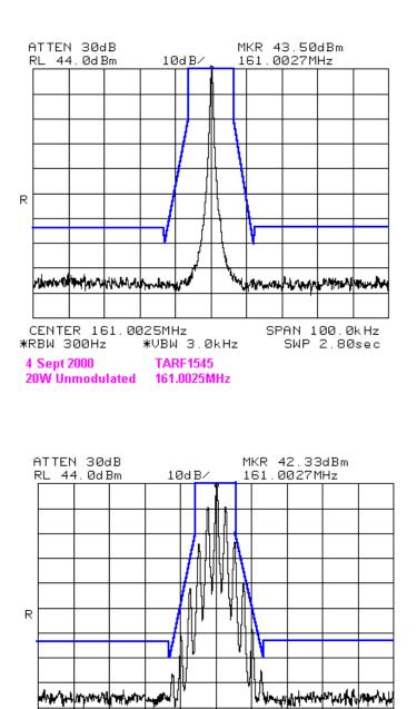
\*RBW 300Hz \*VBW 3.0kHz SWP 2.80sec 4 Sept 2000 TARF1545 20W Modulated 161.0025MHz
