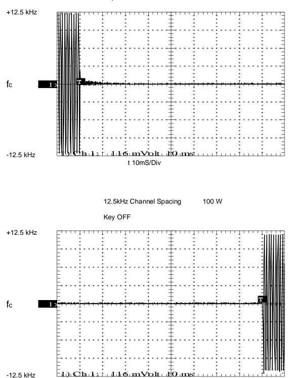
NAME OF TEST: TRANSIENT FREQUENCY BEHAVIOUR
