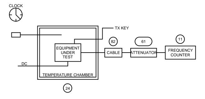
NAME OF TEST: TRANSMITTER FREQUENCY STABILITY
