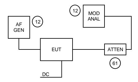
NAME OF TEST: TRANSMITTER MODULATION LIMITING
