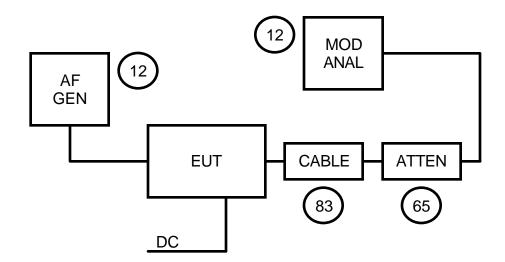
NAME OF TEST: TRANSMITTER AUDIO FREQUENCY RESPONSE
