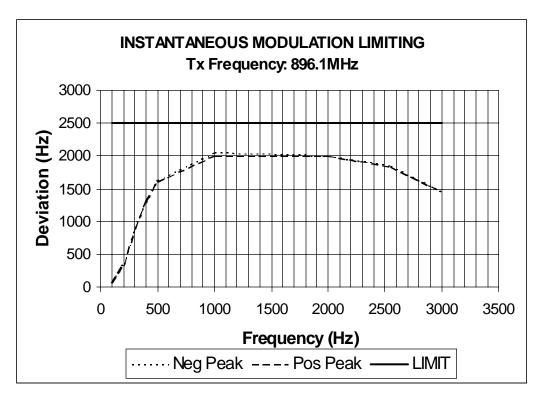
NAME OF TEST: TRANSMITTER MODULATION LIMITING
