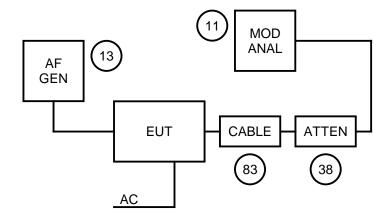
NAME OF TEST: TRANSMITTER AUDIO FREQUENCY RESPONSE
