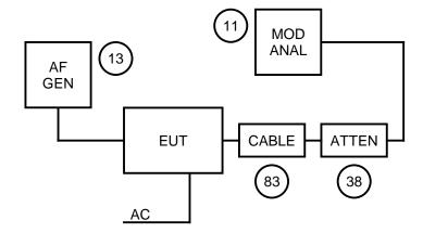
NAME OF TEST: TRANSMITTER MODULATION LIMITING
