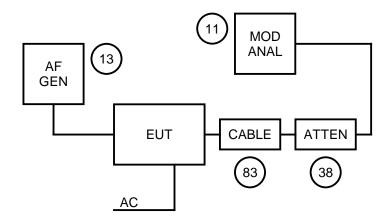
NAME OF TEST: TRANSMITTER MODULATION LIMITING
