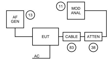
NAME OF TEST: TRANSMITTER MODULATION LIMITING
