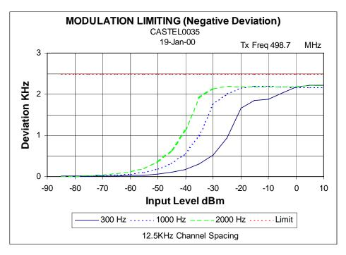
NAME OF TEST: TRANSMITTER MODULATION LIMITING
