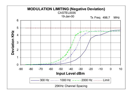
NAME OF TEST: TRANSMITTER MODULATION LIMITING
