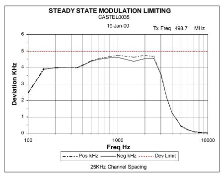
NAME OF TEST: TRANSMITTER MODULATION LIMITING
