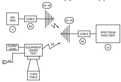
NAME OF TEST: SPURIOUS EMISSIONS (RADIATED)
