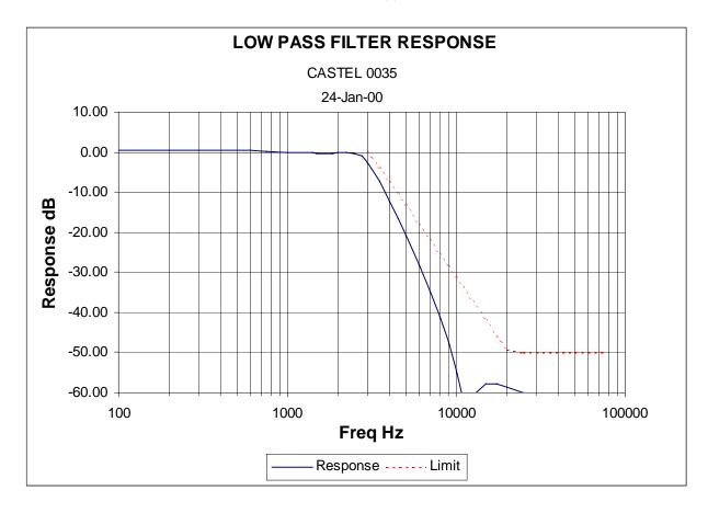
NAME OF TEST: TRANSMITTER AUDIO FREQUENCY RESPONSE
