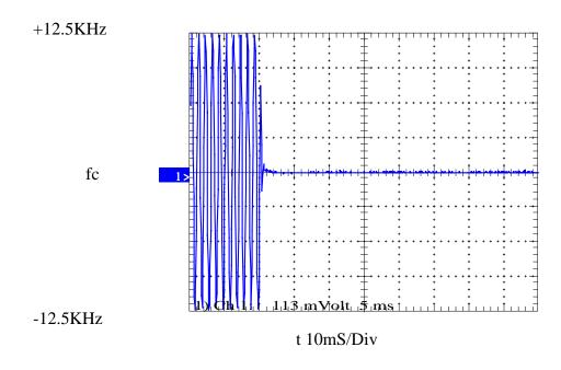
12.5KHz CHANNEL SPACING 100W KEY-OFF
