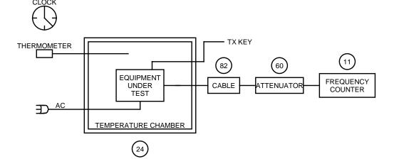
NAME OF TEST: TRANSMITTER FREQUENCY STABILITY
