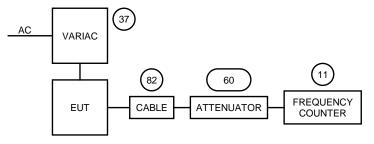
NAME OF TEST:TRANSIENT FREQUENCY BEHAVIORTEST CONDITIONS:Ambient temperature 21 °C<br/>Relative humidity 60 %<br/>Standard Voltage 120VACSPECIFICATION:FCC 47 CFR 90.214GUIDE:TIA/EIA-603 2.2.19
