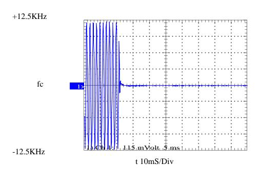
12.5KHz CHANNEL SPACING 20W KEY-OFF
