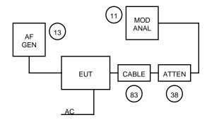
NAME OF TEST: TRANSMITTER AUDIO FREQUENCY RESPONSE
