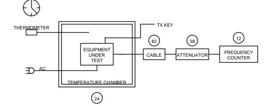
NAME OF TEST: TRANSMITTER FREQUENCY STABILITY (TEMPERATURE)
