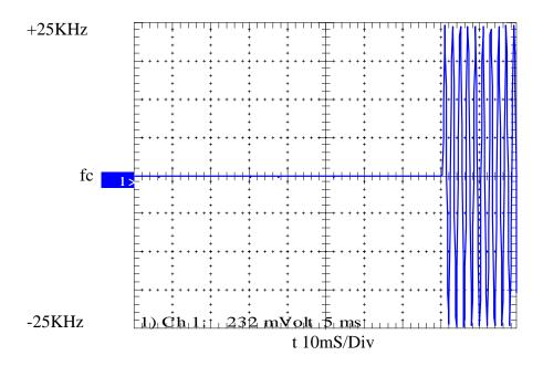
NAME OF TEST: TRANSIENT FREQUENCY BEHAVIOUR
