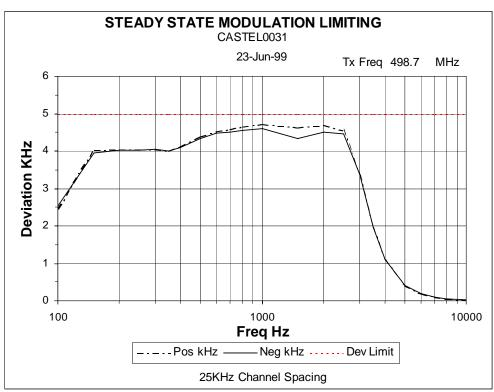
NAME OF TEST: TRANSMITTER MODULATION LIMITING
