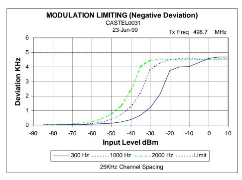
NAME OF TEST: TRANSMITTER MODULATION LIMITING
