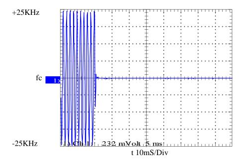
25KHz CHANNEL SPACING 10W KEY-OFF
