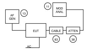
NAME OF TEST: TRANSMITTER MODULATION LIMITING
