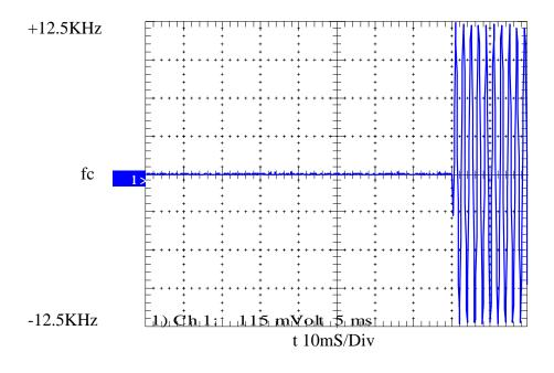
NAME OF TEST: TRANSIENT FREQUENCY BEHAVIOUR
