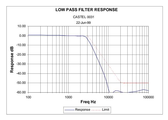
NAME OF TEST: TRANSMITTER AUDIO FREQUENCY RESPONSE
