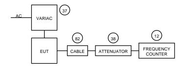
NAME OF TEST: TRANSIENT FREQUENCY BEHAVIOUR
