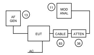
NAME OF TEST: TRANSMITTER MODULATION LIMITING
