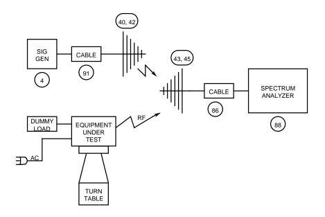
NAME OF TEST: SPURIOUS EMISSIONS (RADIATED)
