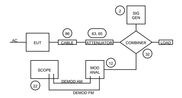
NAME OF TEST: TRANSIENT FREQUENCY BEHAVIOUR
