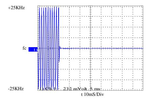
25KHz CHANNEL SPACING 50W KEY-OFF
