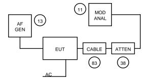
NAME OF TEST: TRANSMITTER MODULATION LIMITING
