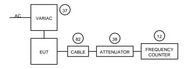
NAME OF TEST: TRANSIENT FREQUENCY BEHAVIOUR
