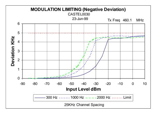
NAME OF TEST: TRANSMITTER MODULATION LIMITING STEADY STATE
