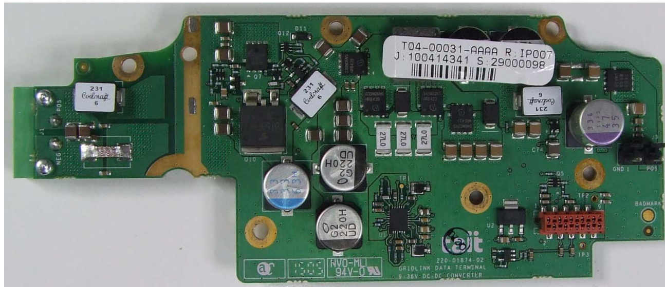
Photograph 08: DC-DC PCB top
