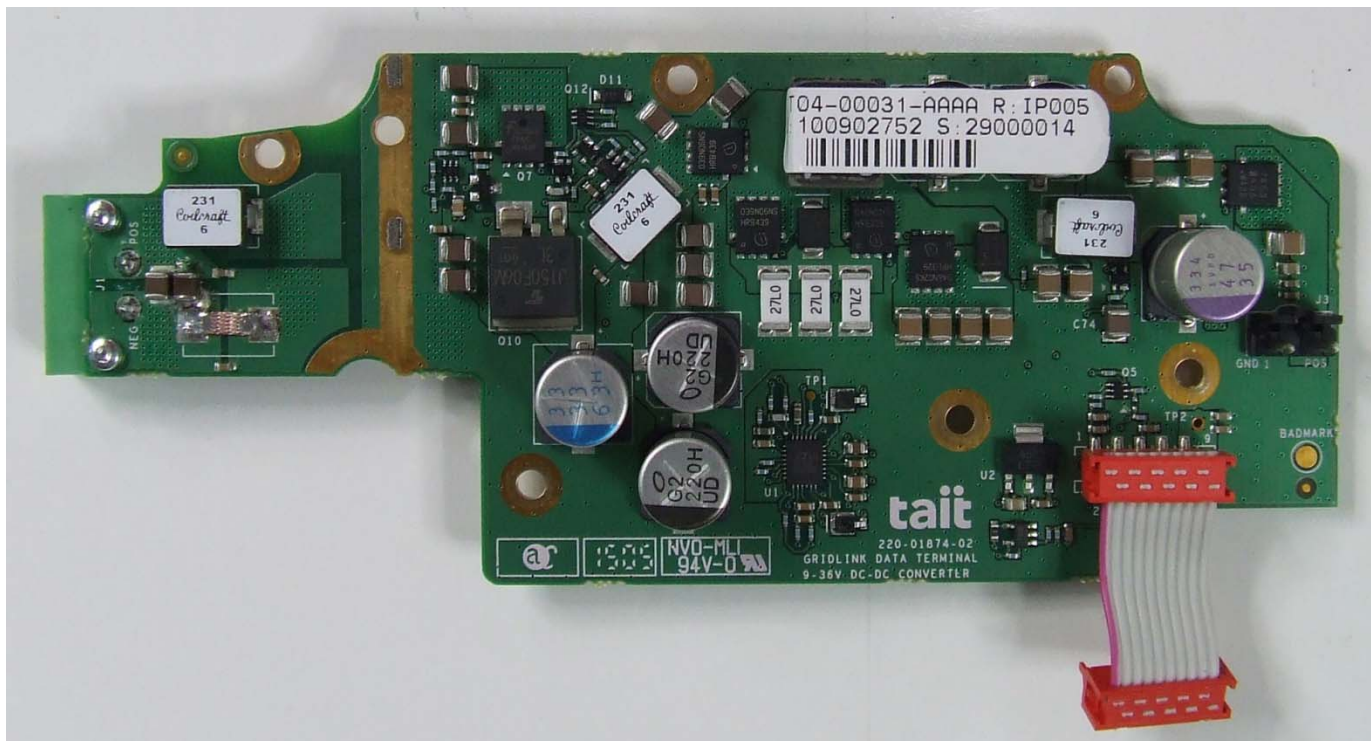
Photograph 08: DC-DC PCB top
