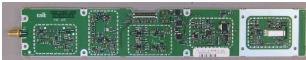
Photograph 21: Transmit Forward Power Board (TXF) – Top (cans off)
