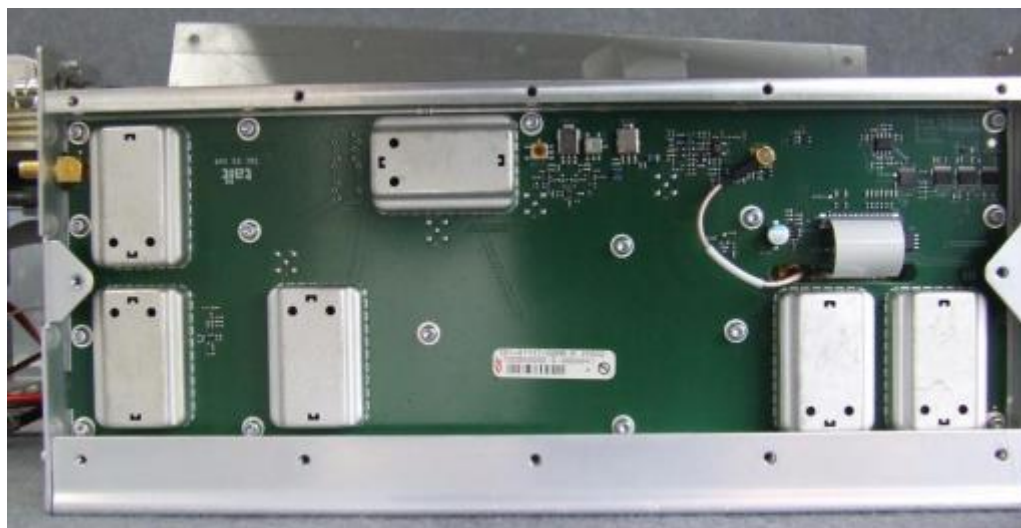
Photograph 17: Receiver Board (RXB) – Top
