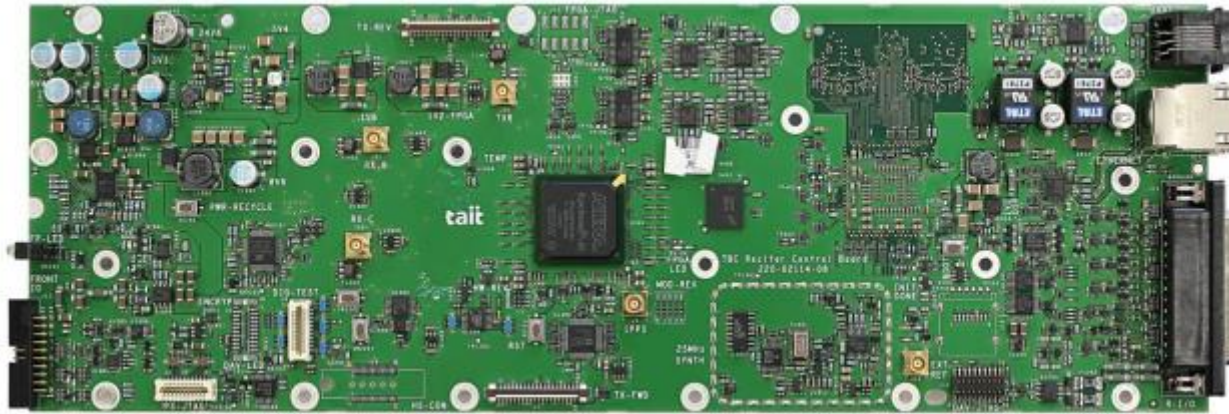
Photograph 15: Reciter Control Board (RCB) – Top (can off)
