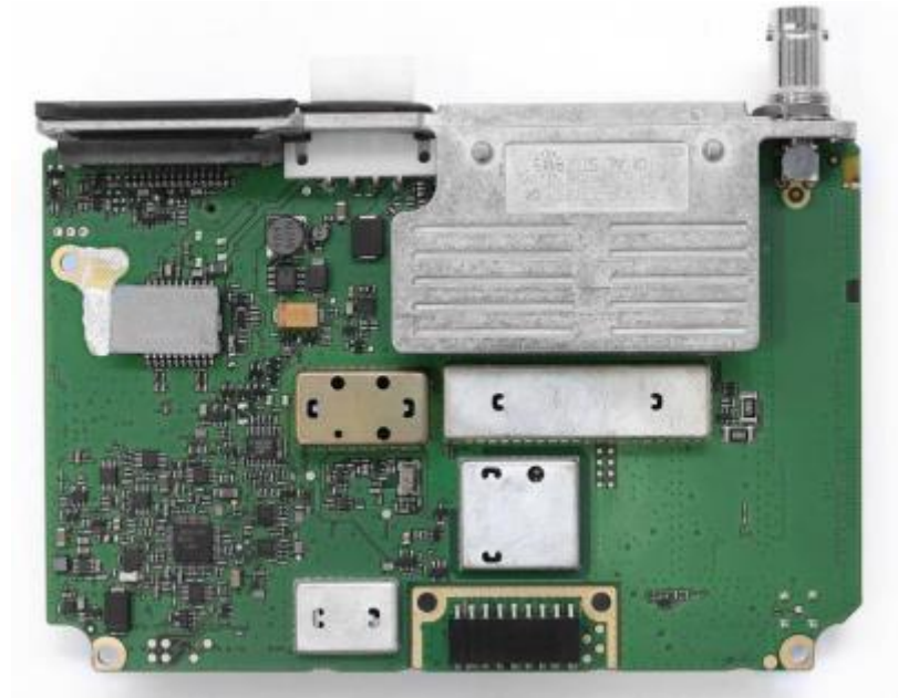
Photograph 13: Power Amplifier PCB – Bottom
