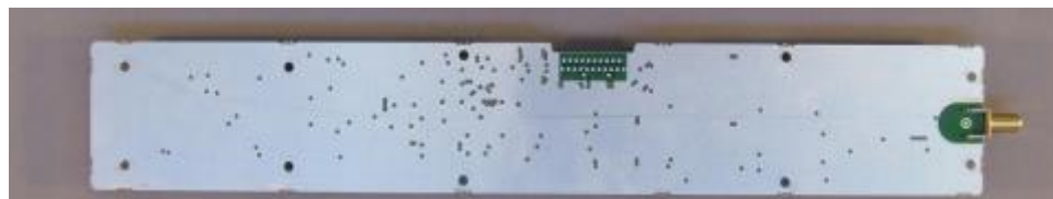
Photograph 22: Transmit Forward Power Board (TXF) – Bottom
