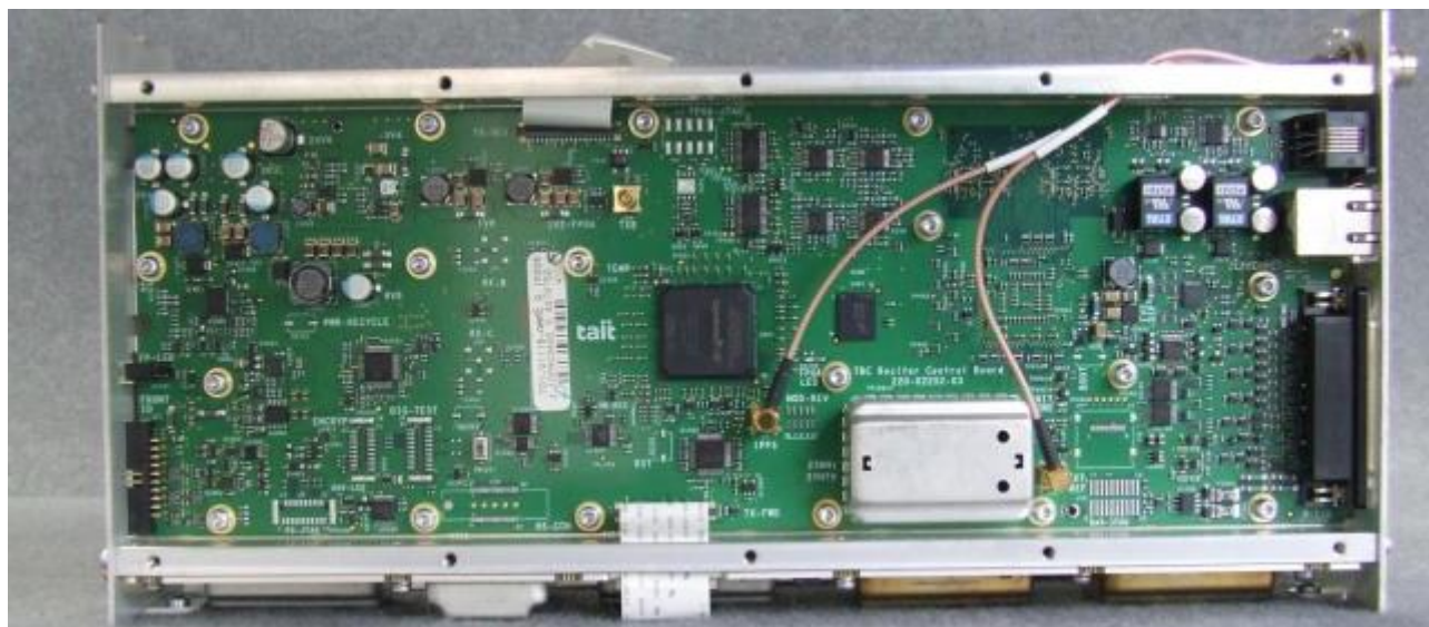
Photograph 14: Reciter Control Board (RCB) – Top
