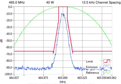
P25 Ph1-C4FM 465.0000MHz Mask D 40W RBW=100Hz, VBW=1000Hz, Detector Mode=Peak Result=Pass
