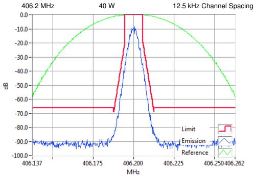
P25 Ph1-C4FM 406.2000MHz Mask D 40W RBW=100Hz, VBW=1000Hz, Detector Mode=Peak Result=Pass
