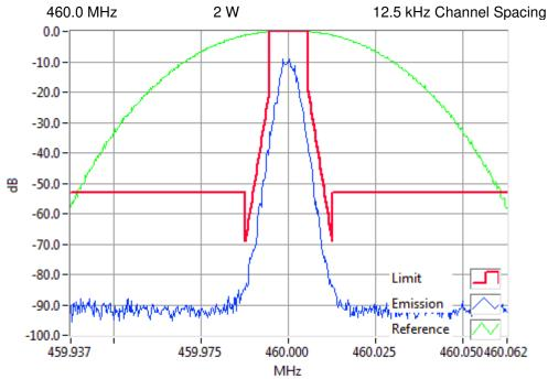
P25 Ph1-C4FM 460.0000MHz Mask D 2W RBW=100Hz, VBW=1000Hz, Detector Mode=Peak Result=Pass
