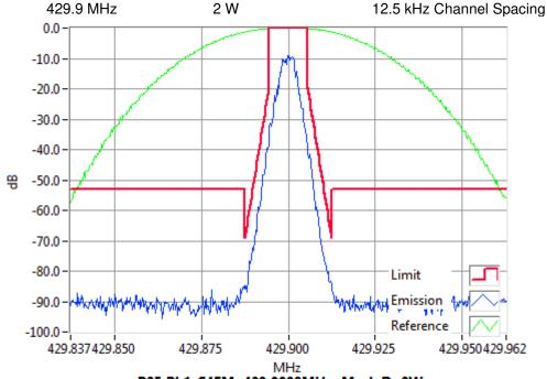
P25 Ph1-C4FM 429.9000MHz Mask D 2W RBW=100Hz, VBW=1000Hz, Detector Mode=Peak Result=Pass
