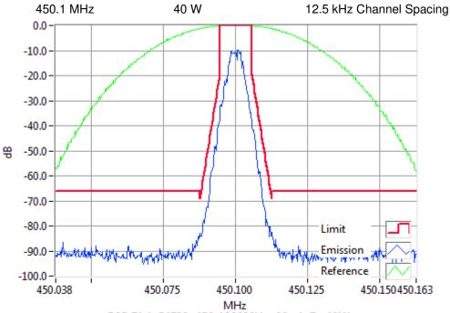
P25 Ph1-C4FM 450.1000MHz Mask D 40W RBW=100Hz, VBW=1000Hz, Detector Mode=Peak Result=Pass
