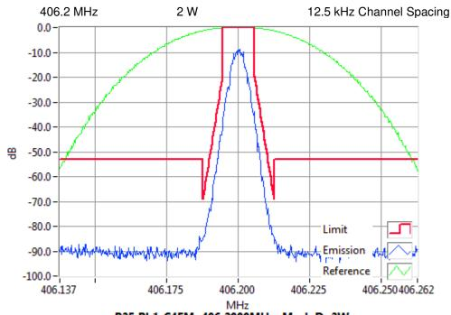
P25 Ph1-C4FM 406.2000MHz Mask D 2W RBW=100Hz, VBW=1000Hz, Detector Mode=Peak Result=Pass
