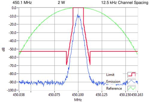
P25 Ph1-C4FM 450.1000MHz Mask D 2W RBW=100Hz, VBW=1000Hz, Detector Mode=Peak Result=Pass
