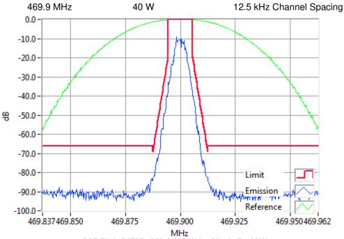
P25 Ph1-C4FM 469.9000MHz Mask D 40W RBW=100Hz, VBW=1000Hz, Detector Mode=Peak Result=Pass
