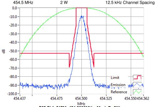
P25 Ph1-C4FM 454.5000MHz Mask D 2W RBW=100Hz, VBW=1000Hz, Detector Mode=Peak Result=Pass
