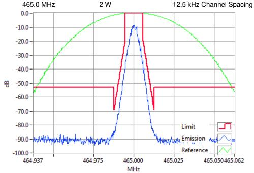
P25 Ph1-C4FM 465.0000MHz Mask D 2W RBW=100Hz, VBW=1000Hz, Detector Mode=Peak Result=Pass
