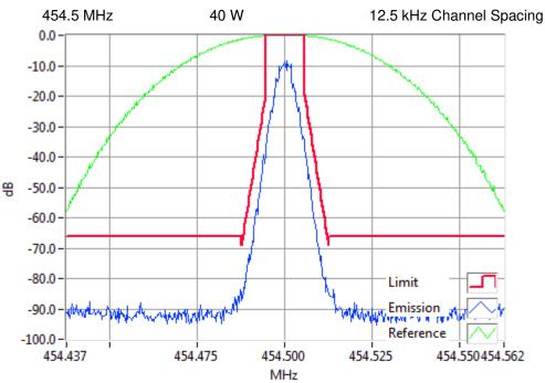
P25 Ph1-C4FM 454.5000MHz Mask D 40W RBW=100Hz, VBW=1000Hz, Detector Mode=Peak Result=Pass
