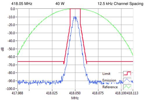
P25 Ph1-C4FM 418.0500MHz Mask D 40W RBW=100Hz, VBW=1000Hz, Detector Mode=Peak Result=Pass
