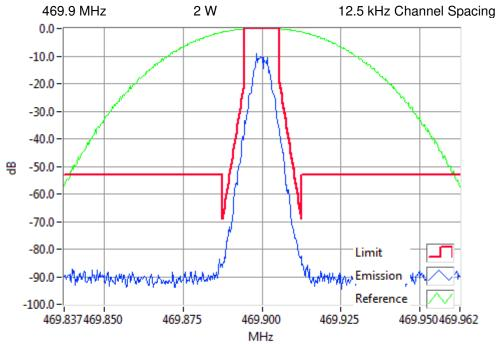
P25 Ph1-C4FM 469.9000MHz Mask D 2W RBW=100Hz, VBW=1000Hz, Detector Mode=Peak Result=Pass
