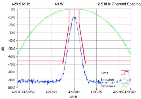
P25 Ph1-C4FM 429.9000MHz Mask D 40W RBW=100Hz, VBW=1000Hz, Detector Mode=Peak Result=Pass
