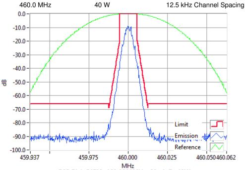
P25 Ph1-C4FM 460.0000MHz Mask D 40W RBW=100Hz, VBW=1000Hz, Detector Mode=Peak Result=Pass
