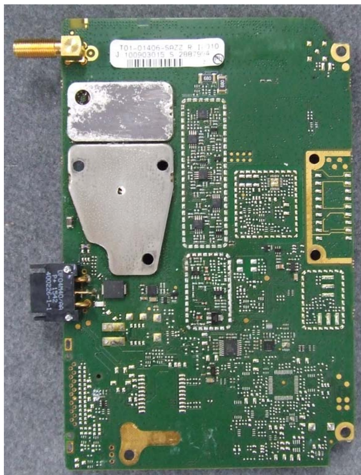
Photograph 09: Power Amplifier PCB – Bottom, cans off
