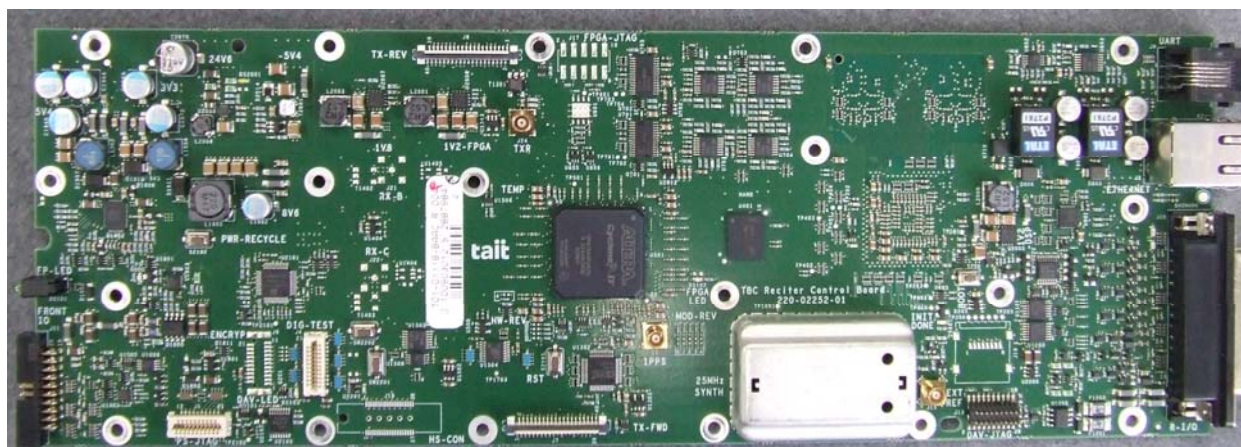
Photograph 10: Reciter Control Board (RCB) – Top
