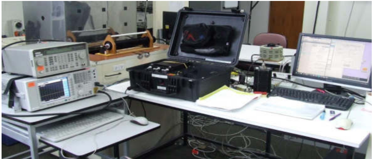
Photo: Conducted Emissions Test Setup
