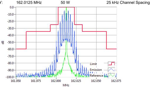
Analogue Modulation 162.0125MHz Mask B 50W RBW=300Hz, VBW=3000Hz, Detector Mode=Peak Result=Pass
