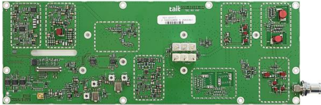
Photograph 18: Receiver Board (RXB) – Top (cans off)
