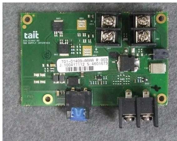
Photograph 09: Supply Interface PCB - Top
