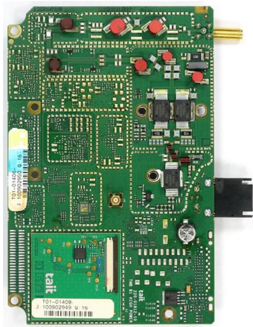
Photograph 12: Power Amplifier PCB – Top, cans off
