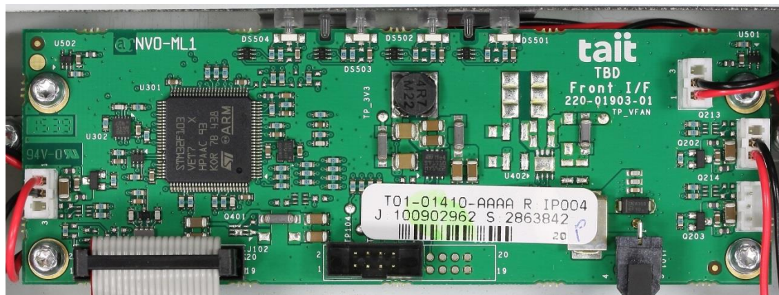
Photograph 07: Front Interface PCB - Top
