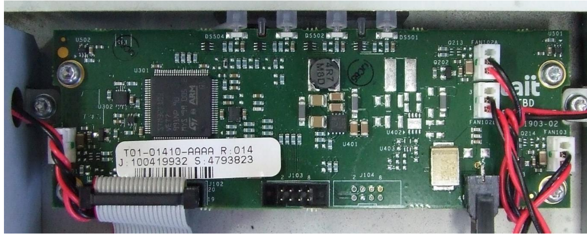
Photograph 03: Front Interface PCB - Top
