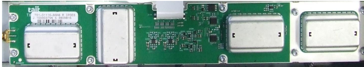
Photograph 21: Transmit Forward Power Board (TXF) – Top
