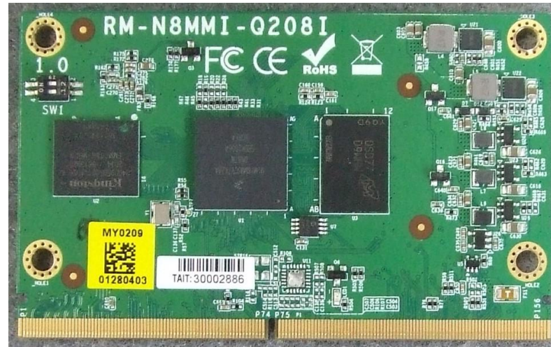
Photograph 15: RCB Smarc Module – Top
