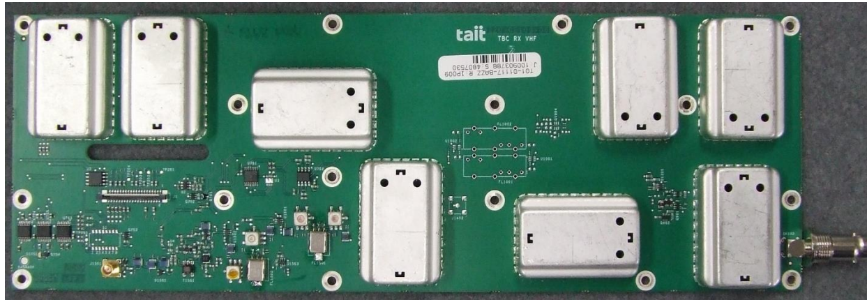
Photograph 18: Receiver Board (RXB) – Top
