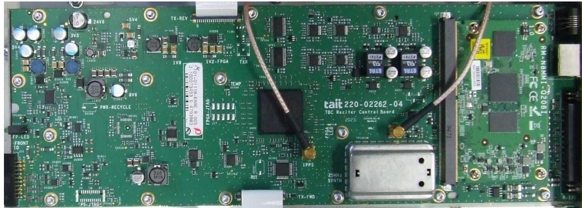
Photograph 13: Reciter Control Board (RCB) – Top
