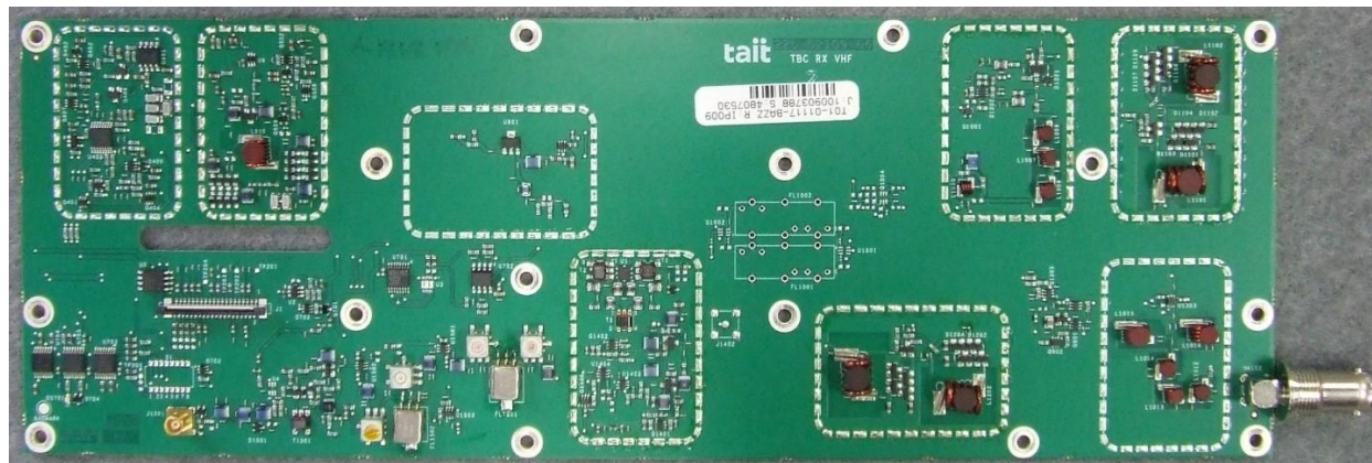
Photograph 19: Receiver Board (RXB) – Top (cans off)
