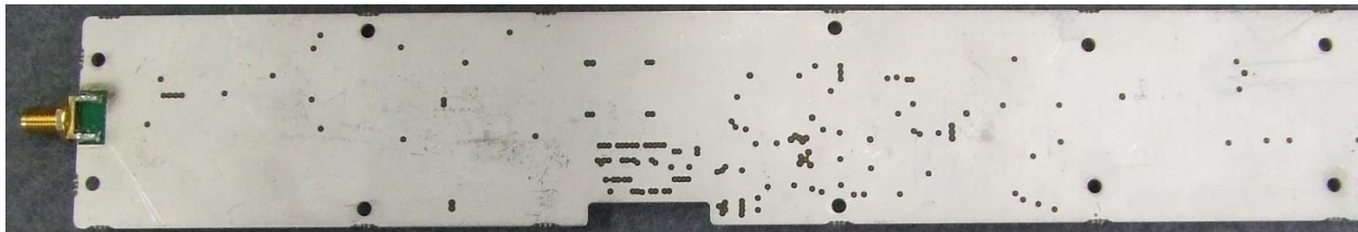
Photograph 23: Transmit Forward Power Board (TXF) – Bottom
