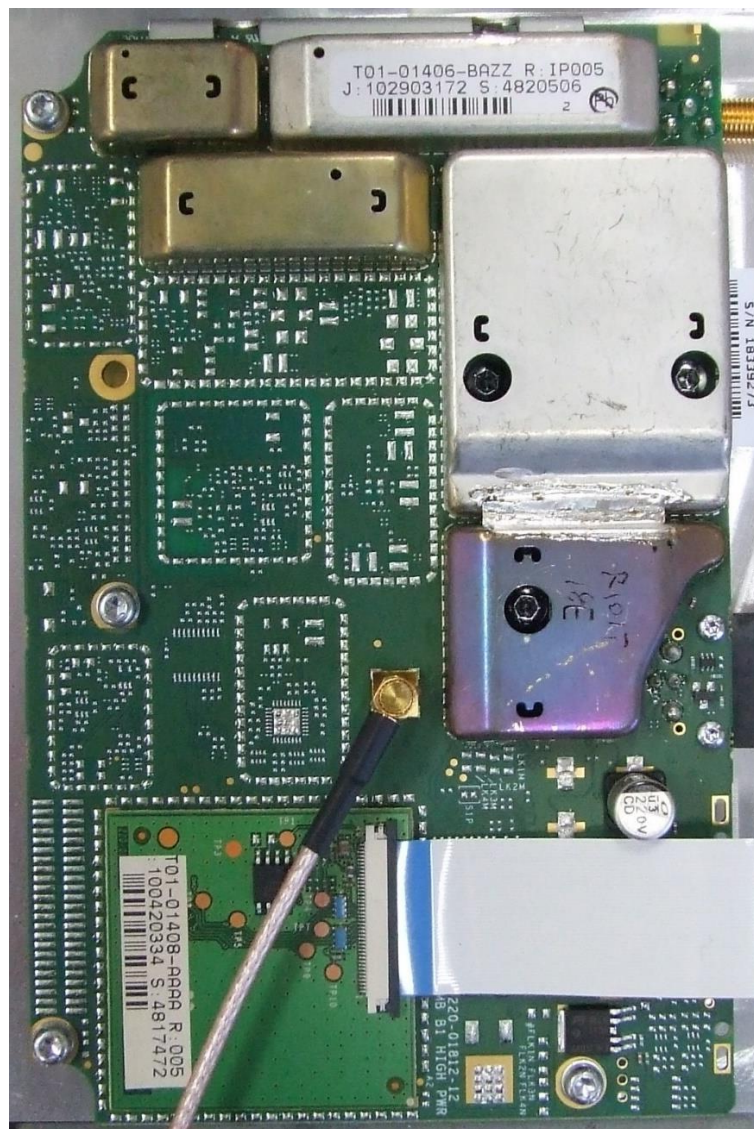
Photograph 09: Power Amplifier PCB – Top
