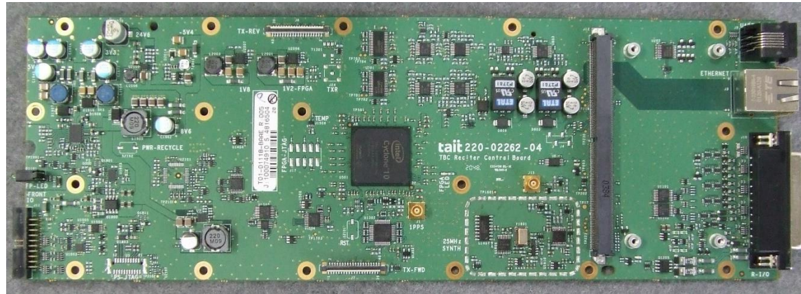
Photograph 14: Reciter Control Board (RCB) – Top (can off)
