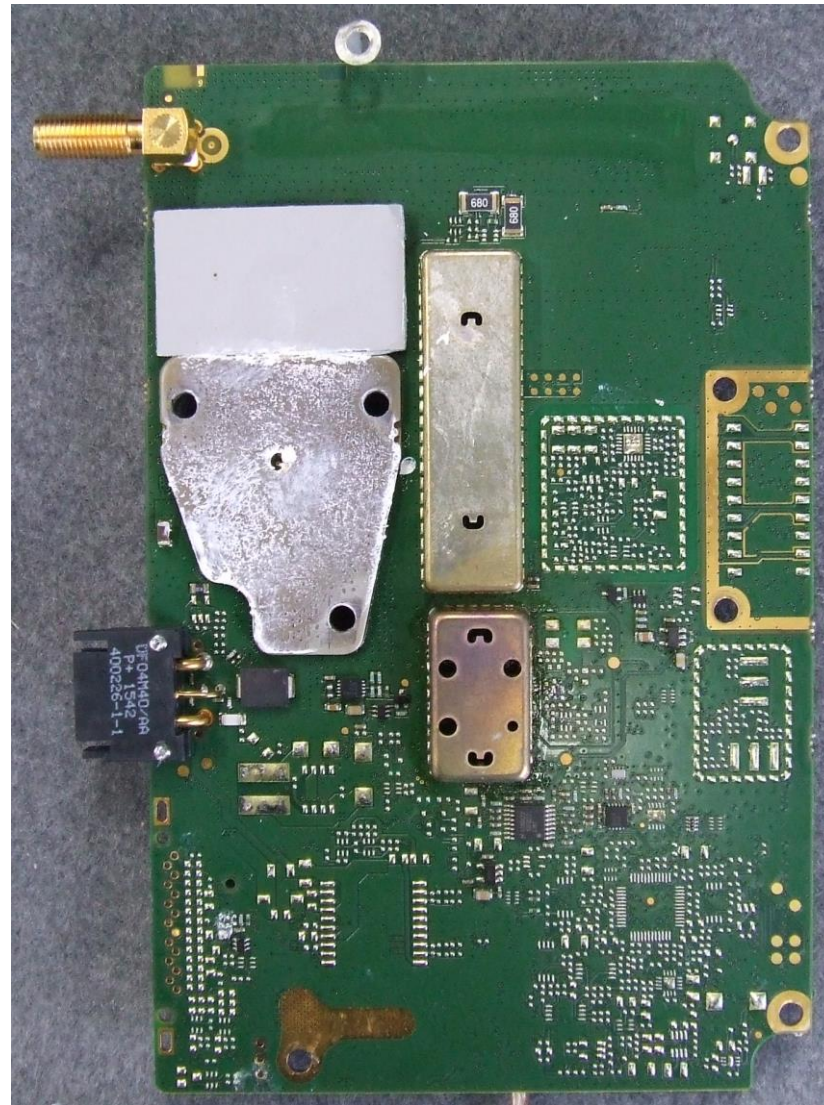
Photograph 11: Power Amplifier PCB – Bottom
