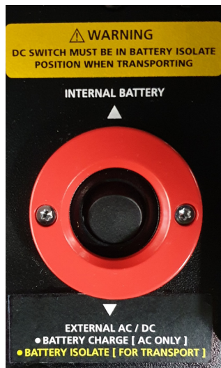
Figure 3.1 Battery select switch
