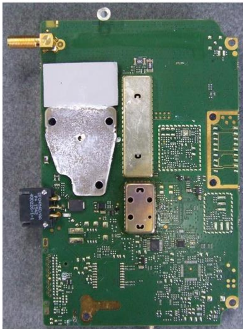
Photograph 13: Power Amplifier PCB – Bottom
