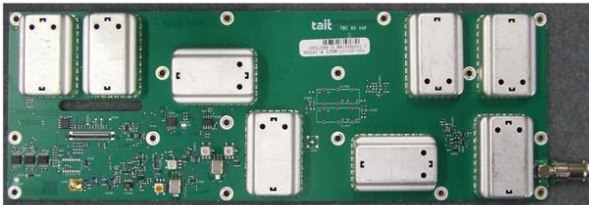
Photograph 18: Receiver Board (RXB) – Top
