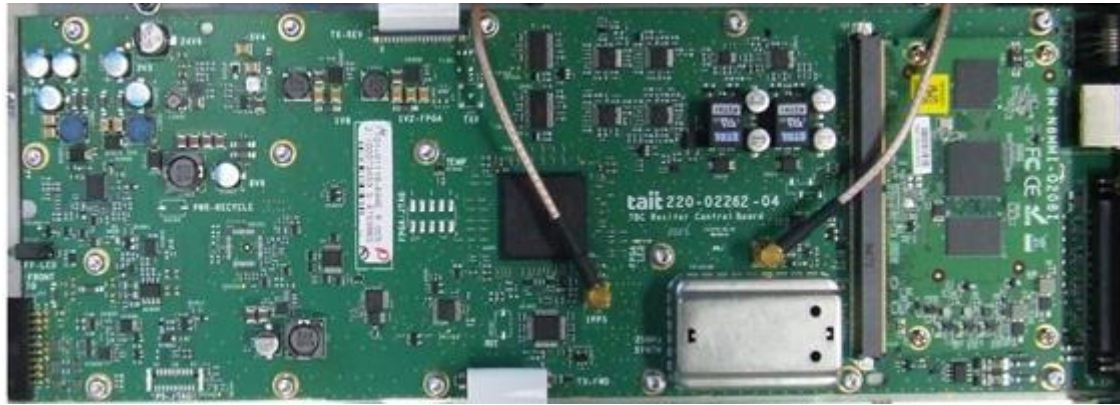
Photograph 15: Reciter Control Board (RCB) – Top
