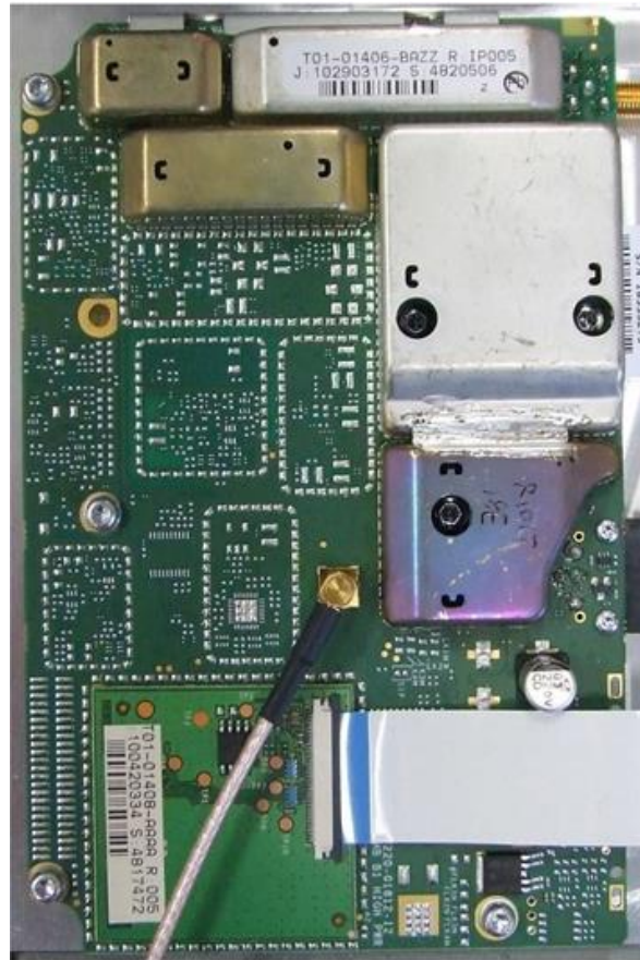
Photograph 11: Power Amplifier PCB – Top
