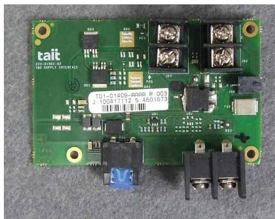
Photograph 09: Supply Interface PCB - Top
