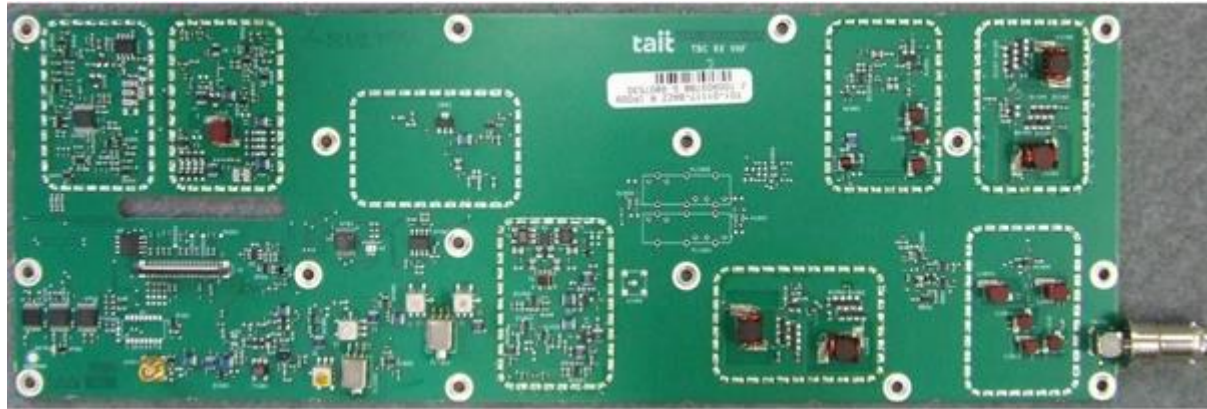
Photograph 19: Receiver Board (RXB) – Top (cans off)
