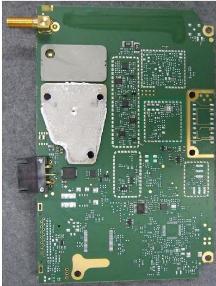
Photograph 14: Power Amplifier PCB – Bottom (can off)
