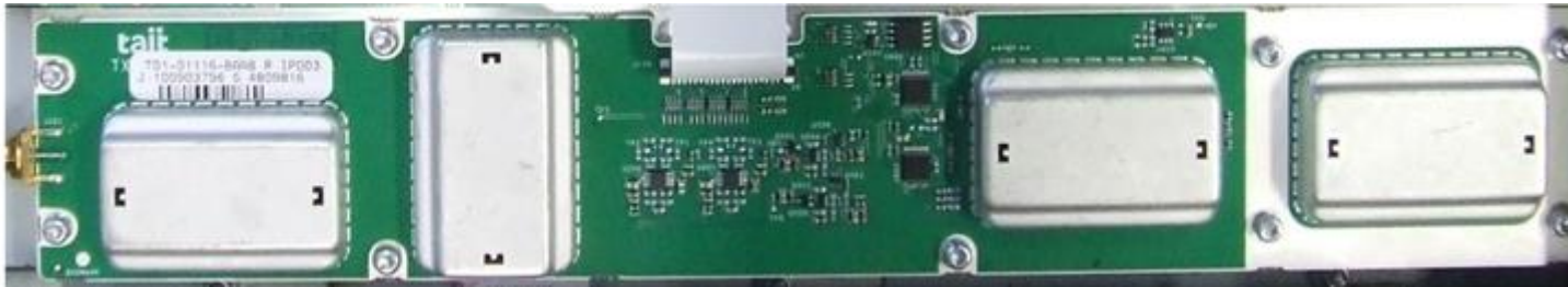
Photograph 21: Transmit Forward Power Board (TXF) – Top
