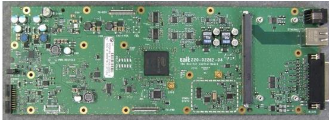
Photograph 16: Reciter Control Board (RCB) – Top (can off)
