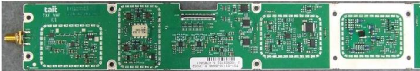
Photograph 22: Transmit Forward Power Board (TXF) – Top (cans off)
