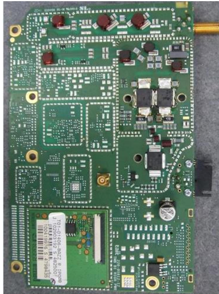
Photograph 12: Power Amplifier PCB – Top, cans off
