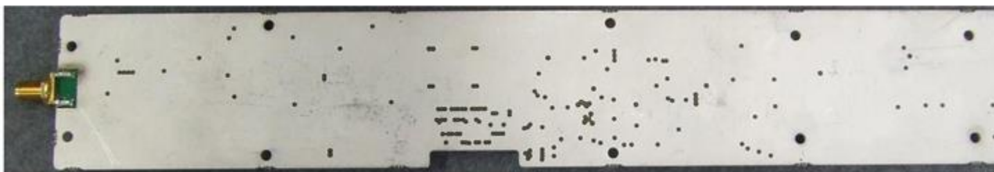
Photograph 22: Transmit Forward Power Board (TXF) – Bottom
