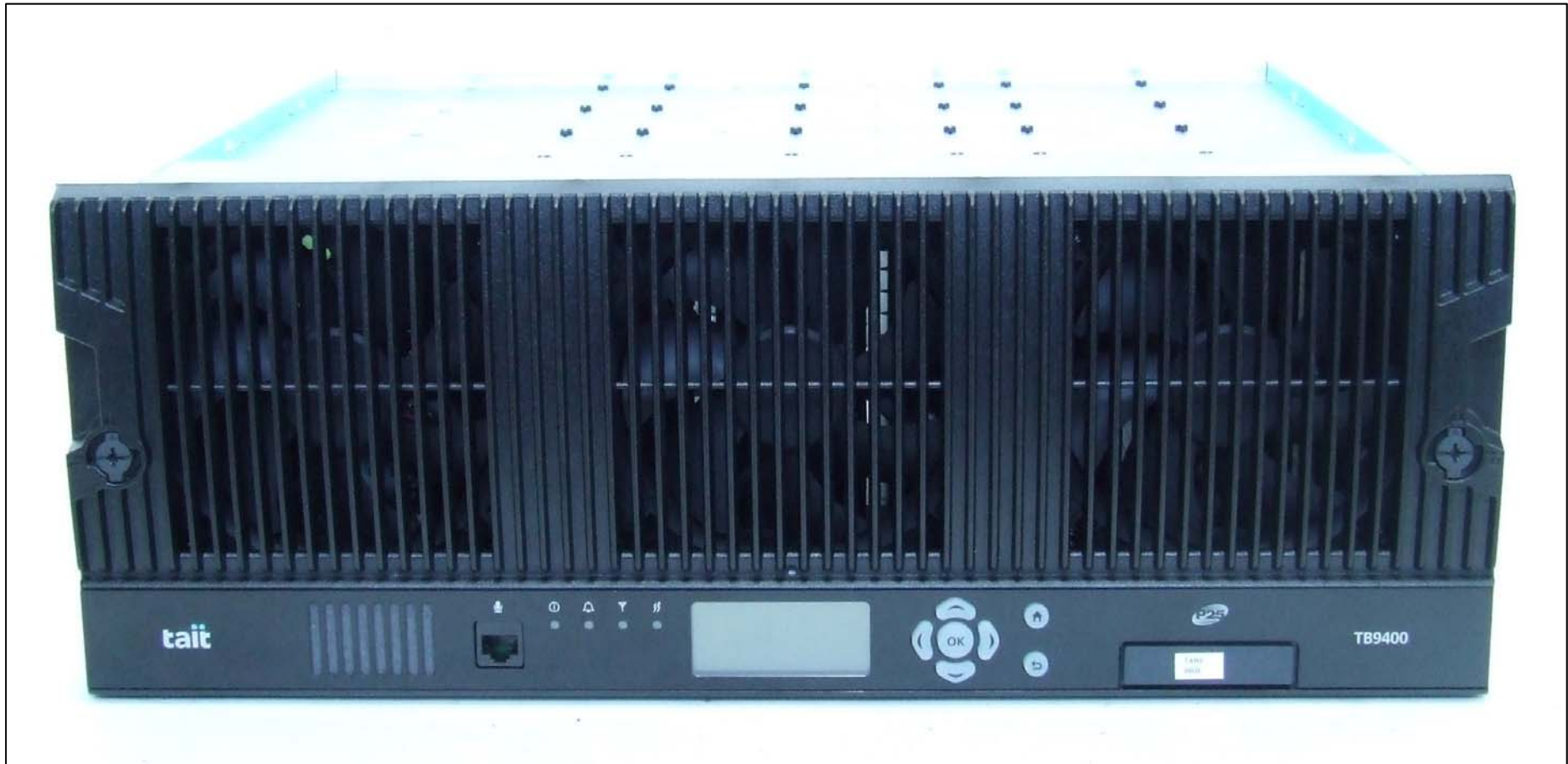
Photograph 02: Rx System – Front panel
