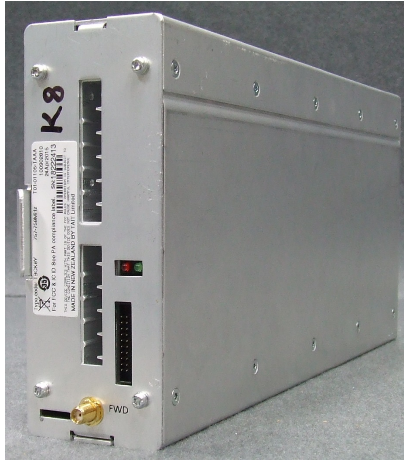
Photograph 01: Reciter module – Product view
