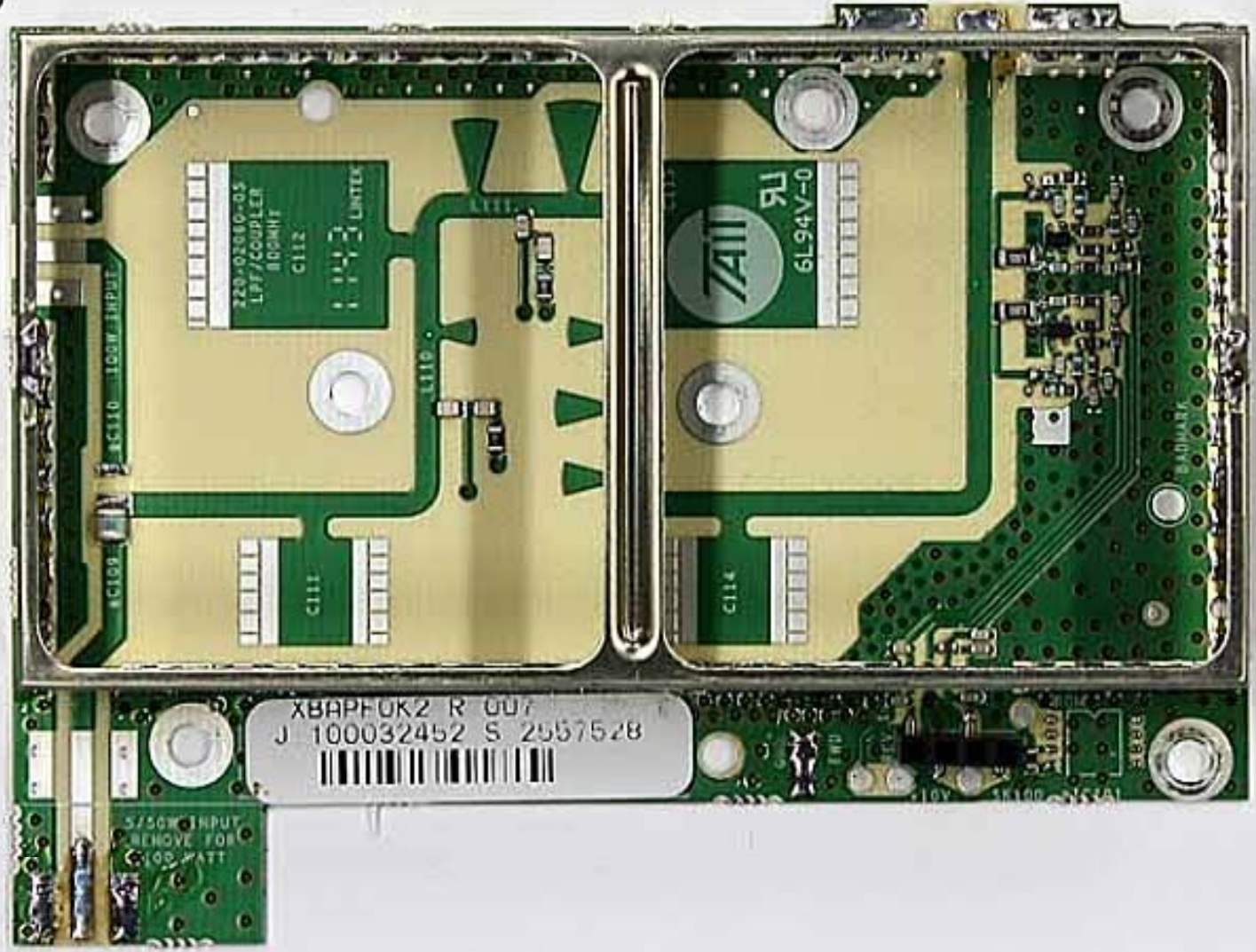
TBCK4D - Internal - Power Amp - LPF - Top - Cans Removed
