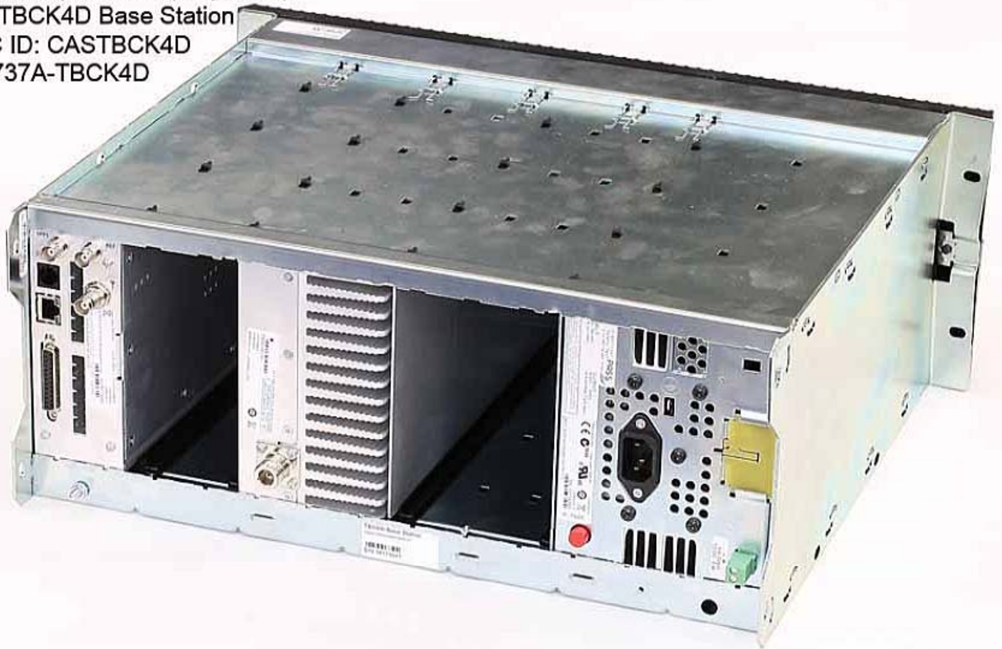
TBCK4D - External - Subrack - Rear/Left Isometric View
