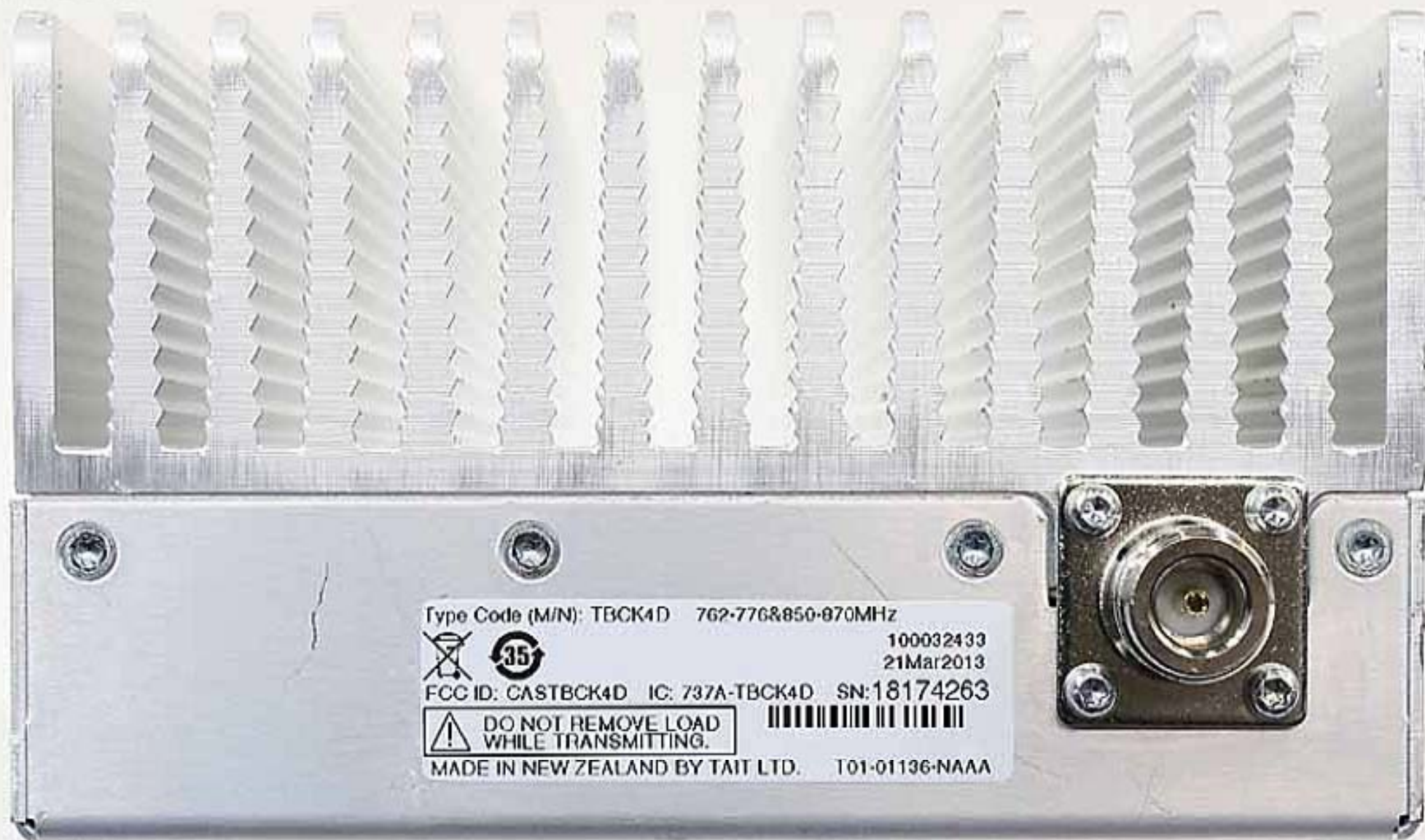
TBCK4D - External - Power Amplifier - Rear (Showing compliance label)
