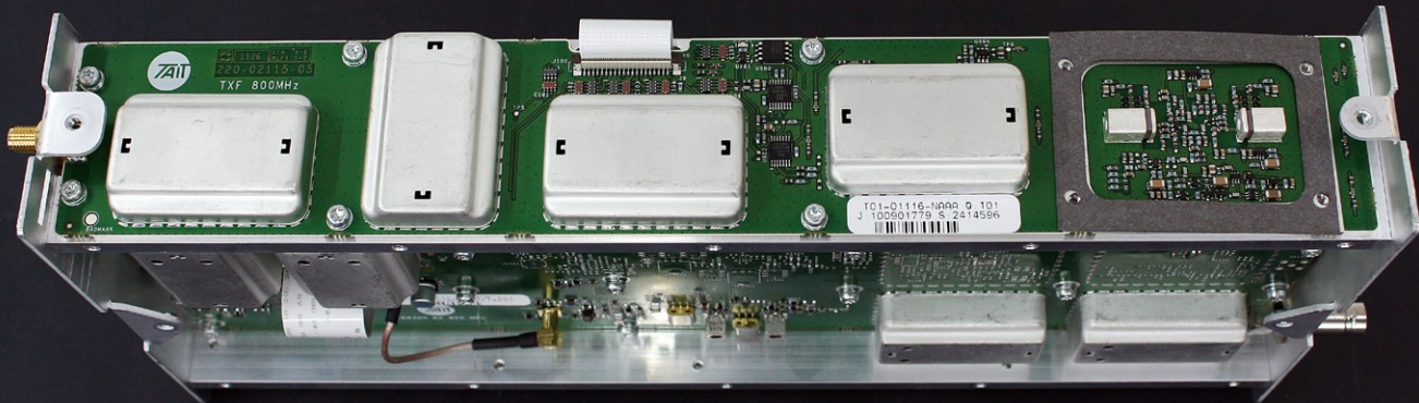
Reciter Transmit Forward Board No Can
