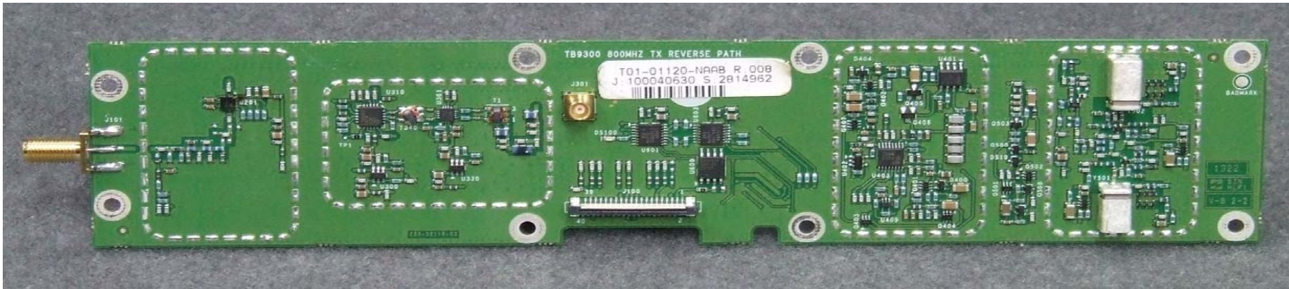
Photograph 14: TXR PCB – Top. Shields Removed
