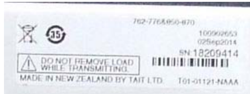
Photograph 03: 50W PA module (762→870MHz) – Compliance label
