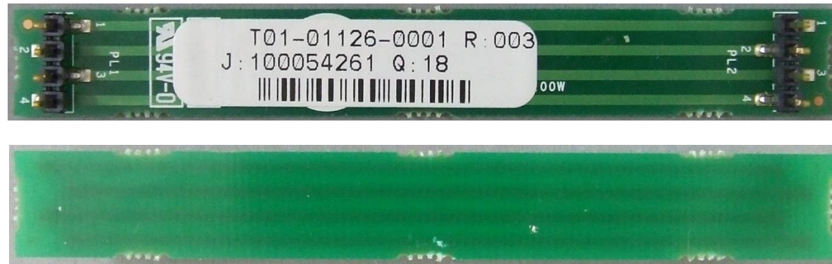
Photograph 27 & 28: Power Amplifier Interconnect PCB – Top & Bottom
