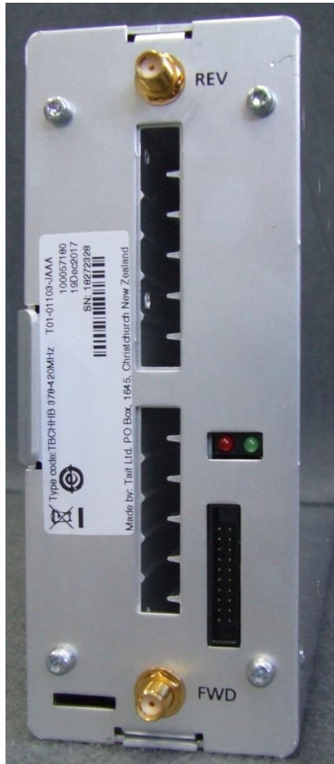
Photograph 06: Reciter module – Front panel
