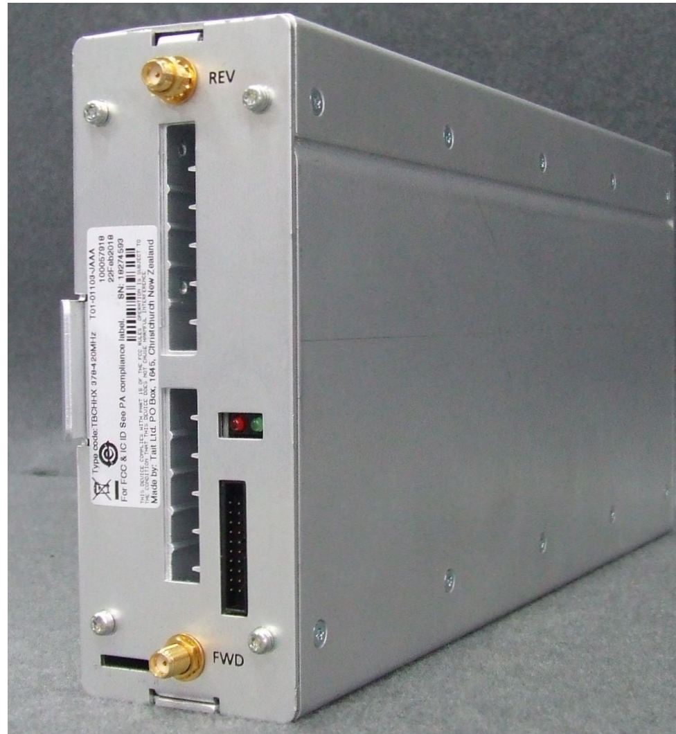
Photograph 05: Reciter module – Product view
