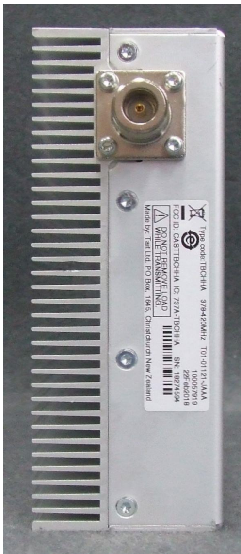
Photograph 10: Power Amplifier – Rear panel
