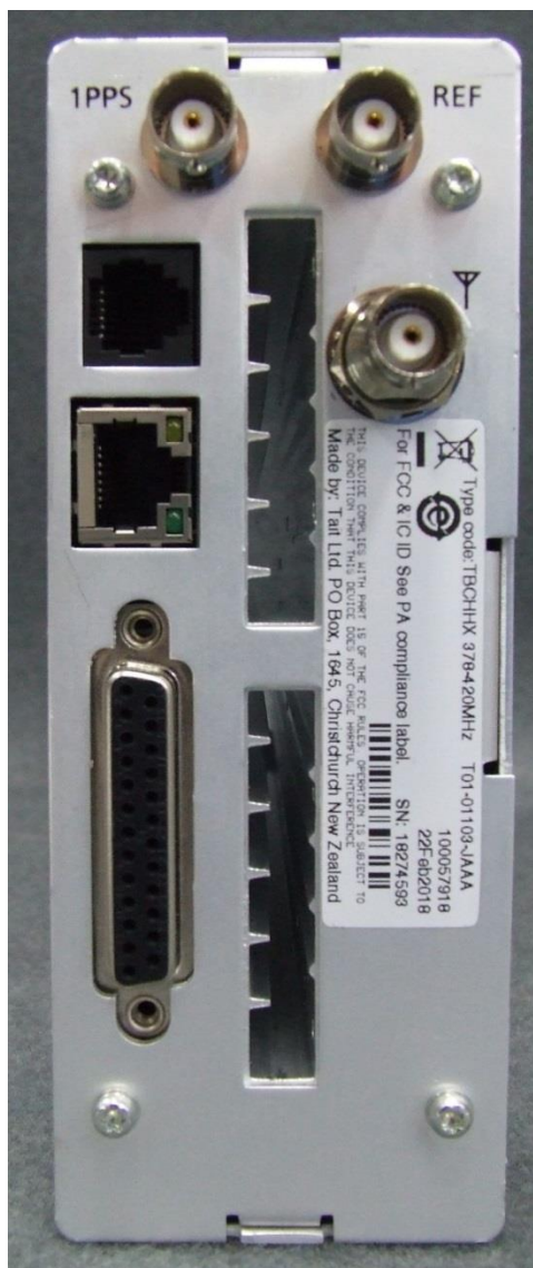
Photograph 07: Reciter module – Rear panel
