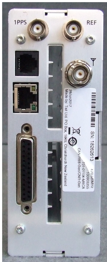
Photograph 07: Reciter module – Rear panel
