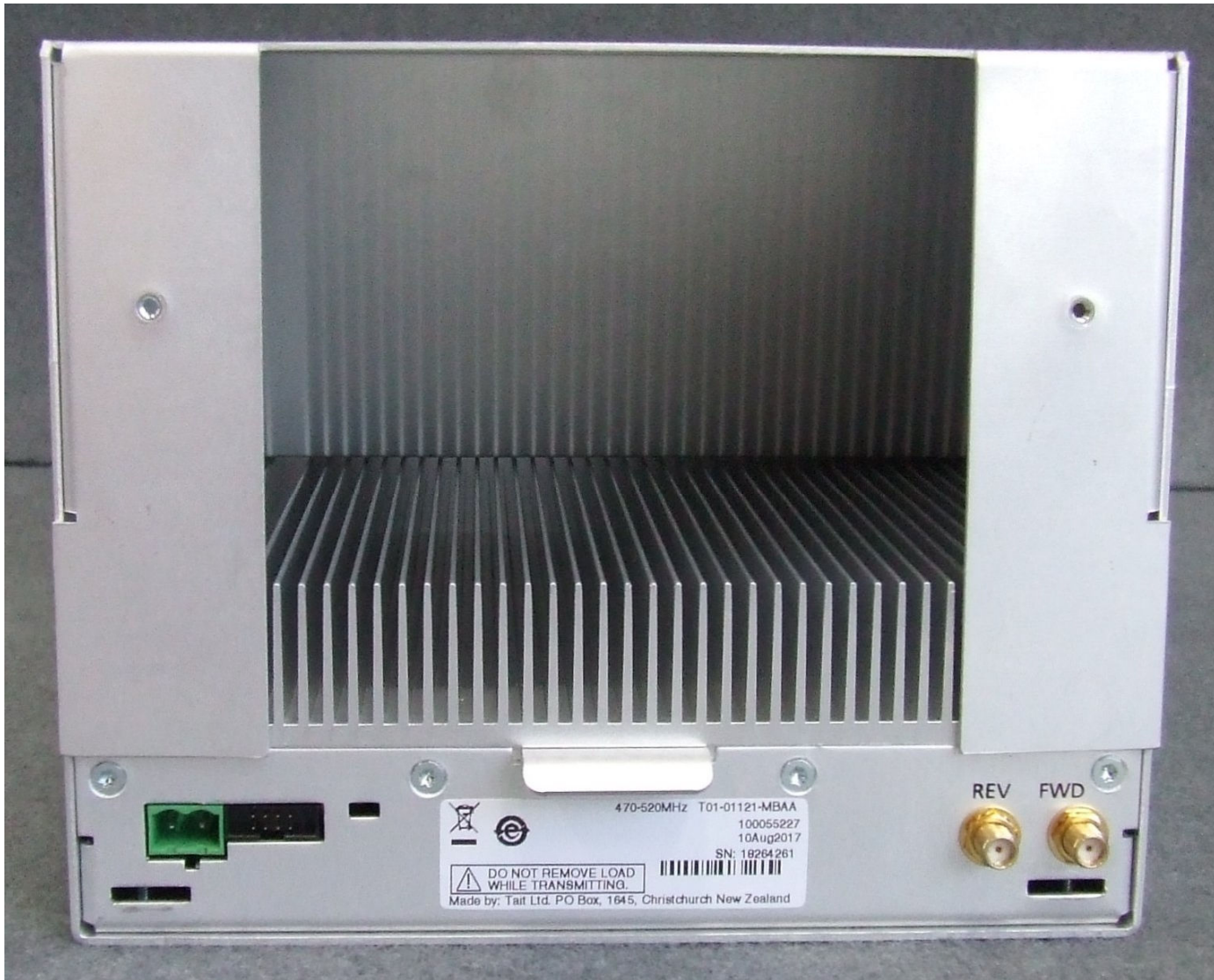
Photograph 09: Power Amplifier – Front panel
