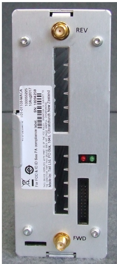
Photograph 06: Reciter module – Front panel
