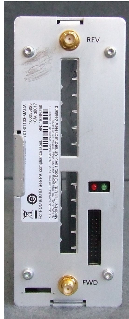
Photograph 06: Reciter module – Front panel
