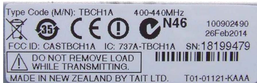
Photograph 03: 50W PA module – Compliance label
