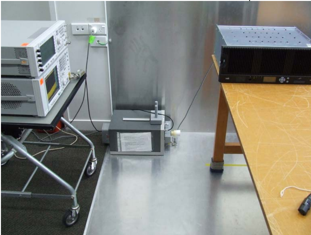
Photo: Power Line Conducted Emissions Test setup
