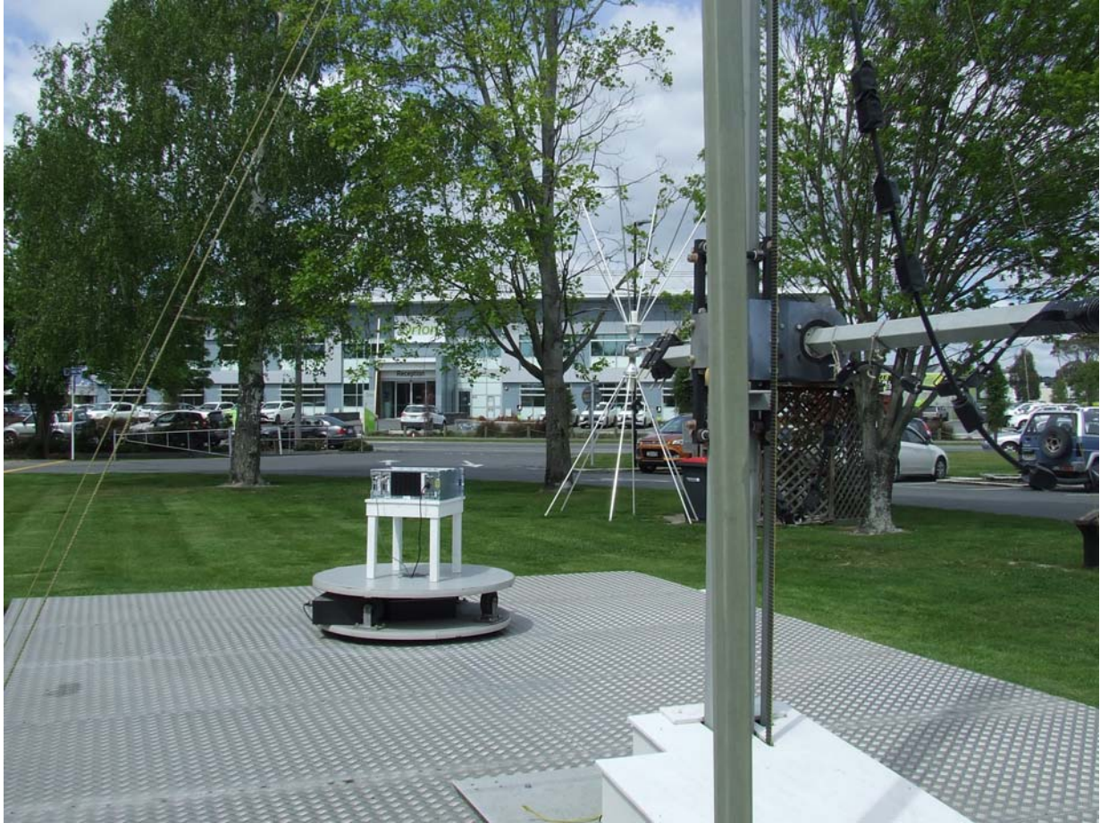
Photo: Radiated Spurious Emissions test setup OATS
