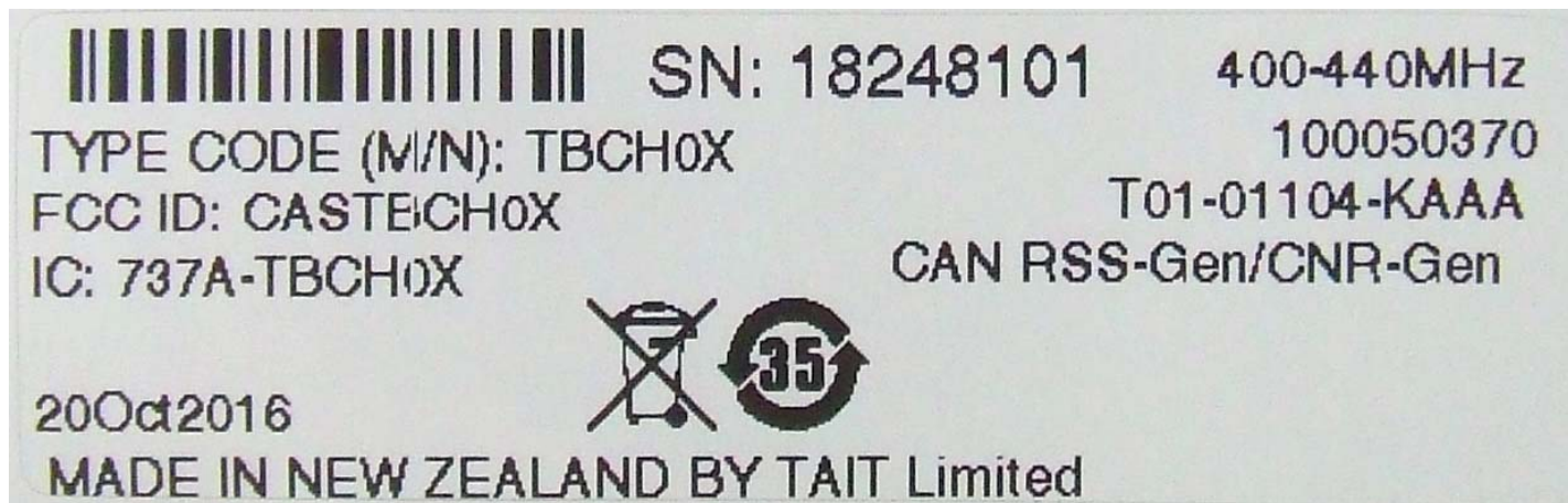
Photograph 02: H1 (400-440 MHz) Reciter module – Compliance label
