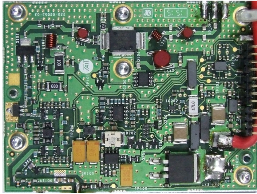
Photograph 14: Power Amplifier 6W Driver PCB – Top & Bottom
