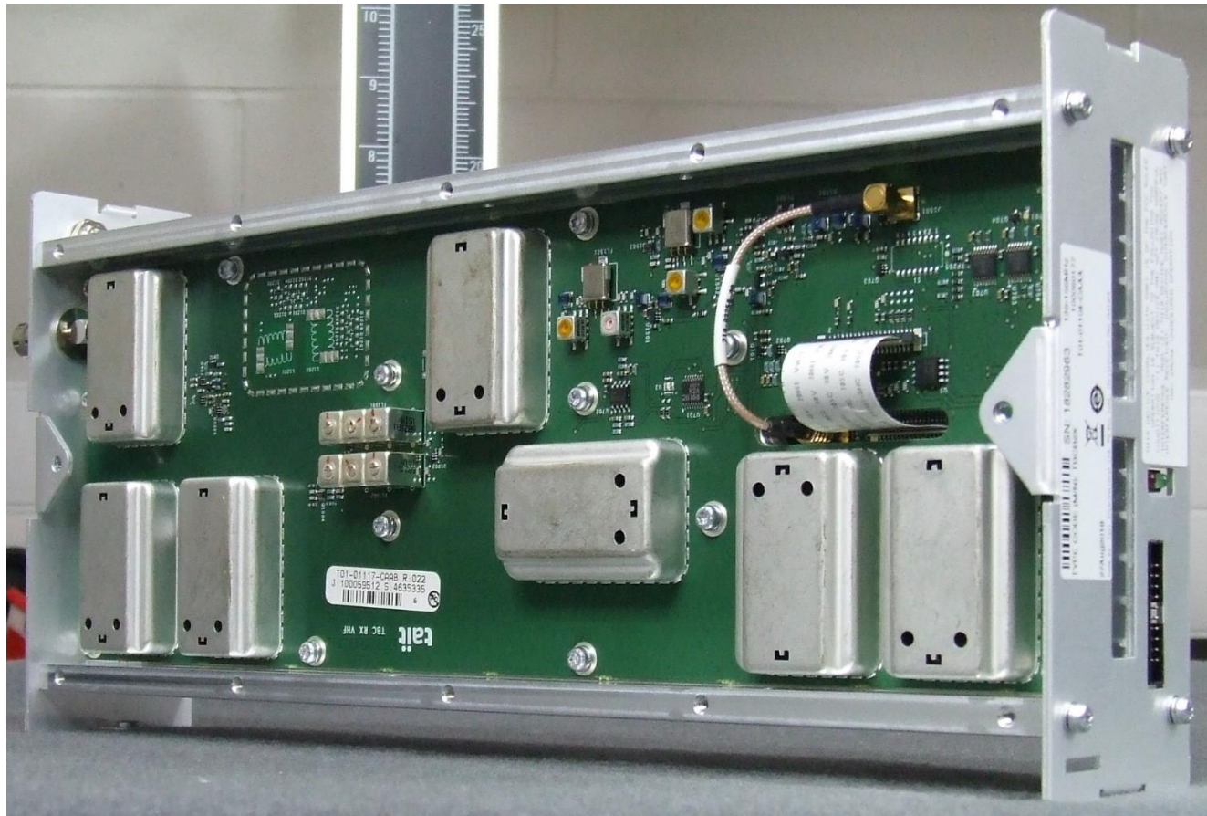
Photograph 01: Reciter module – Internal (Receiver PCB side)
