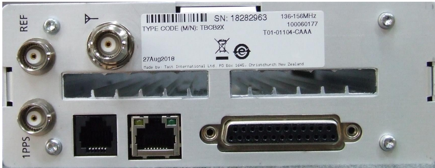
Photograph 07: Reciter module – Rear panel
