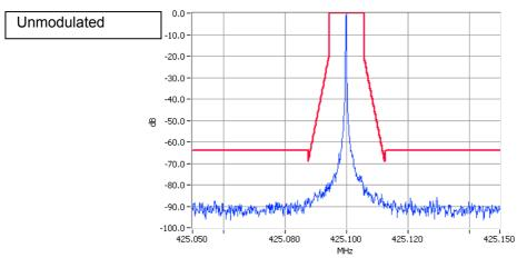
Unmodulated 425.1000MHz Mask D 25W Pass RBW=100Hz VBW=1000Hz
