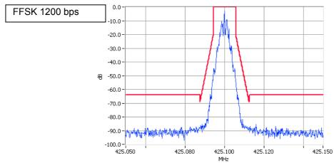
Digital Modulation 425.1000MHz Mask D 25W Pass RBW=100Hz VBW=1000Hz
