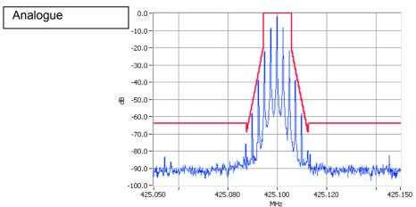
Analogue Modulation 425.1000MHz Mask D 25W Pass RBW=100Hz VBW=1000Hz
