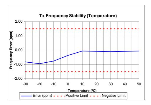
Tx FREQUENCY: 425.1 MHz 25 W 25 kHz channel Spacing
