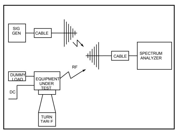
All other testing is performed using the Teltest Radio EVAluation system (TREVA), which is configured as shown below. The Spectrum Analyser is connected to the EUT via the attenuator network for Conducted Emissions testing, and Occupied Bandwidth.
