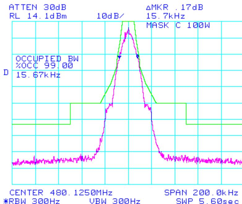
SPECTRUM FOR EMISSION **15K7F1D**, 19200bps, 9600bauds, RC4FSK
