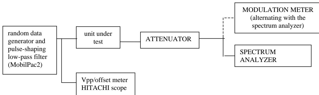
**NAME OF TEST:** Transmitter Occupied Bandwidth
