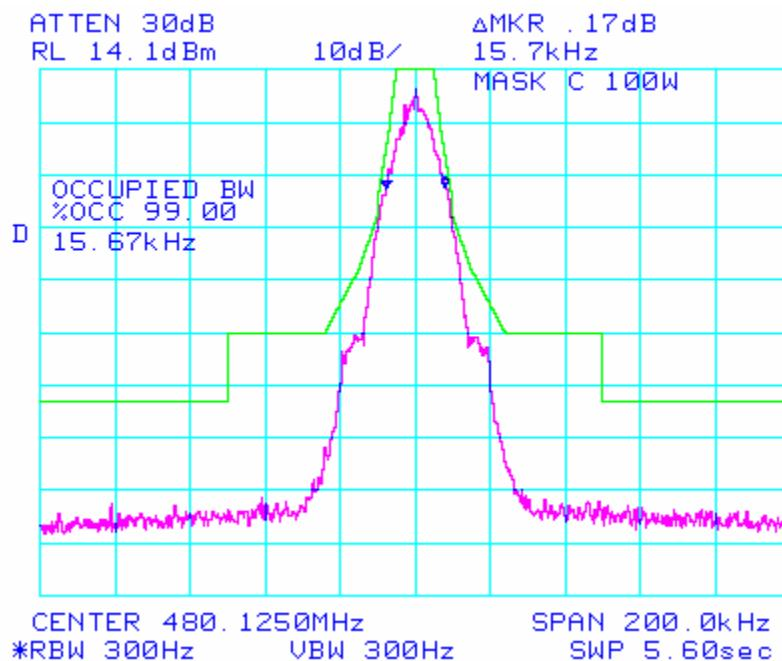
SPECTRUM FOR EMISSION **15K7F1D**, 19200bps, 9600bauds, RC4FSK
