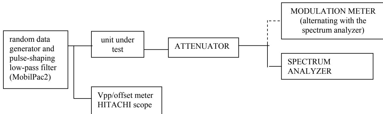
**NAME OF TEST:** Transmitter Occupied Bandwidth
