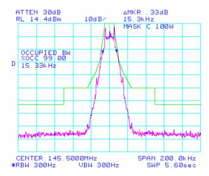
SPECTRUM FOR EMISSION **15K4F1D**, 19200bps, DGMSK BT factor=0.3 PEAK DEVIATION = 4210 Hz, SPAN = 20kHz/div
