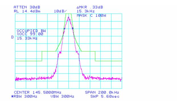
SPECTRUM FOR EMISSION **15K7F1D**, 19200bps, 9600bauds, RC4FSK PEAK DEVIATION = 4840 Hz, SPAN = 20kHz/div
