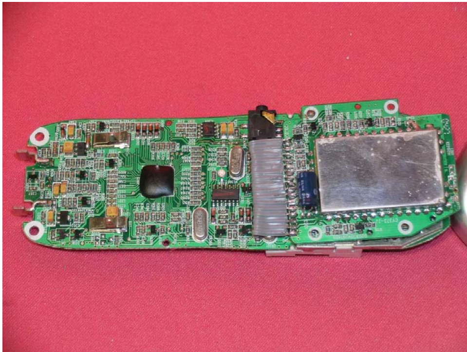
Handset Main PCB comp side (View 1)
