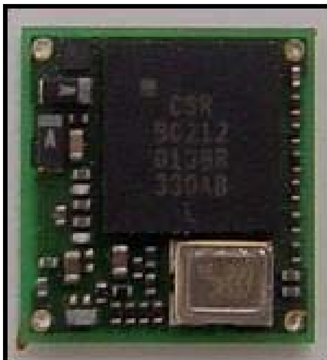
Front View of Bluetooth module without shielding
