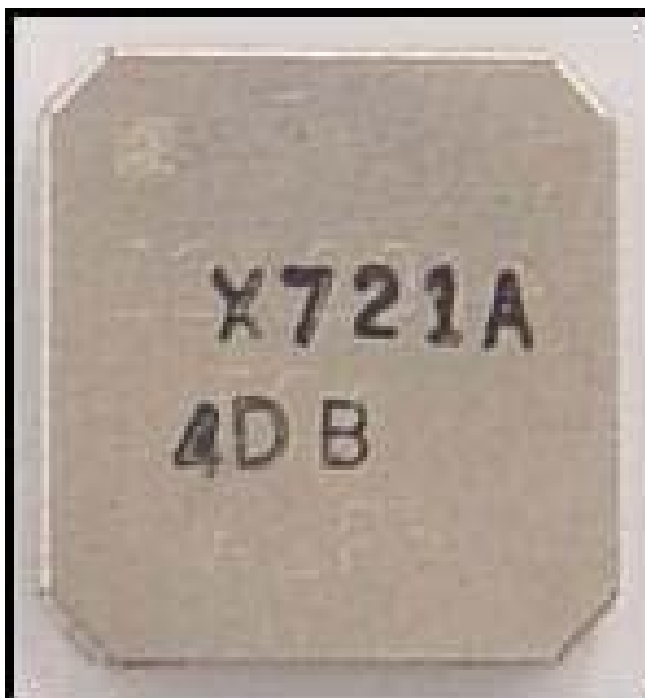
Front View of Bluetooth module without shielding
