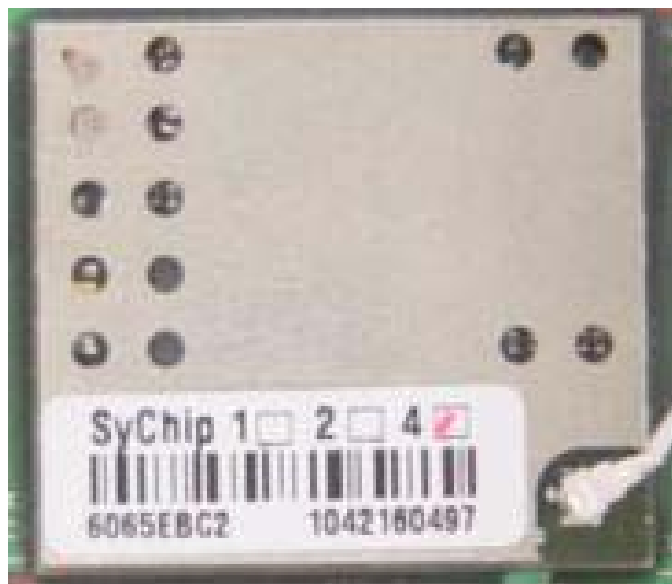
Front View of WLAN module with shielding
