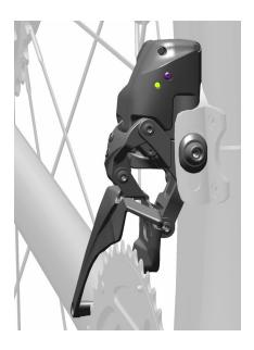
Press and hold the function button on the front derailleur until the green LED blinks quickly, then release.
