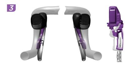
Press both shifter paddles simultaneously to move the front derailleur inboard or outboard.
