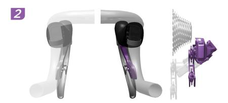
Press the right shifter paddle to move the rear derailleur outboard. Press and hold the paddle for multiple shifts.
