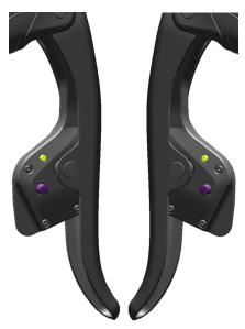
Press and hold the function button on one shifter until the green LED blinks quickly, then release. Repeat on the other shifter.
