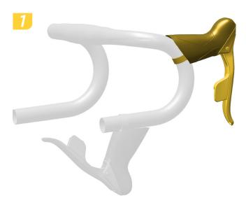
Install the shifter assembly onto the handlebar and set it to your desired position.
