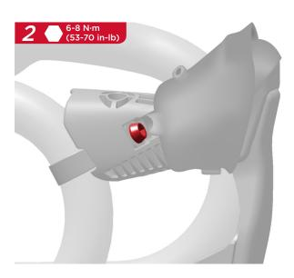
Use a 5 mm hex bit socket to torque the shifter bolt to 6-8 N·m (53-70 in-lbs).
