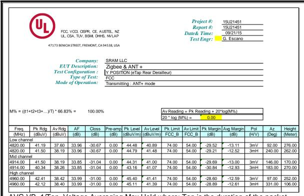
AVG VB=1/Ton, Voltage Averaging Max Hold where: Ton is the duration of the packet
