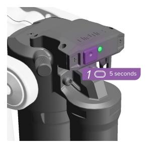
AirWiz must be taken out of Transport mode before it can be used for the first time.
