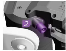
The app will suggest a recommended target air pressure based on your rider weight and bicycle setup, Inflate the fork or shock to the desired pressure. The app will display the current air pressure as you add or release air.
