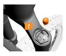
Remove the air valve cap.
