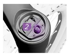
The app will suggest a recommended target air pressure based on your rider weight and bicycle setup, Inflate the fork or shock to the desired pressure. The app will display the current air pressure as you add or release air.
